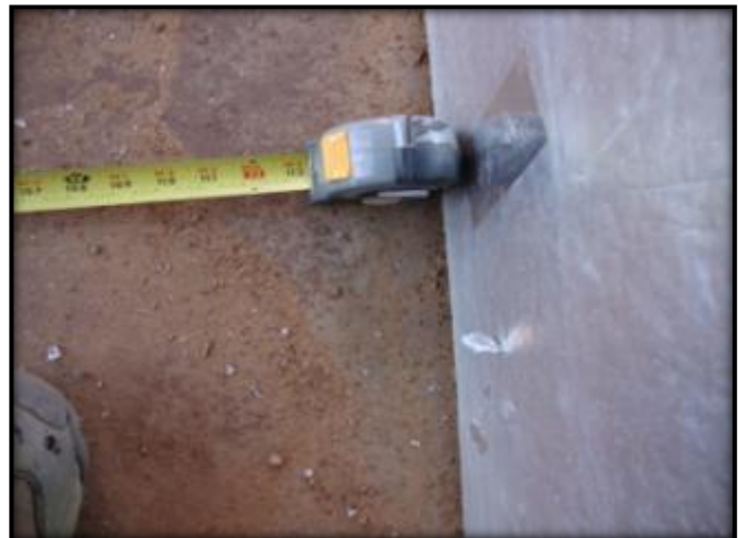
Figure C.20: L5 Fragment In Vertical Witness Panel
