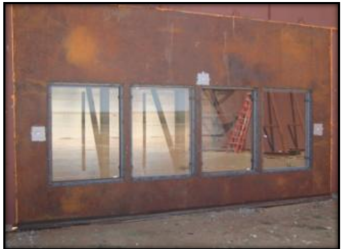
Figure B.4: Pre-Blast Specimen Setup Chamber 2
