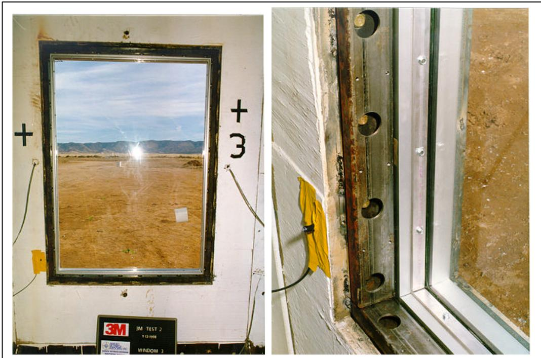
Figure A.67. Test 2. Pretest, interior views of window 3. Close-up view of the batten system shown on right (3M T2 PRE 05.tif, 3M T2 PRE 03.tif).
