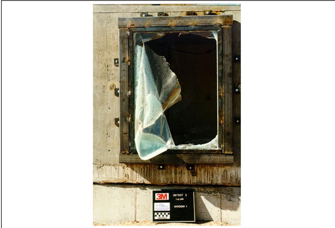
Figure A.153. Test 5. Posttest, exterior view of window 1 (3M T5 POST 26.tif).
