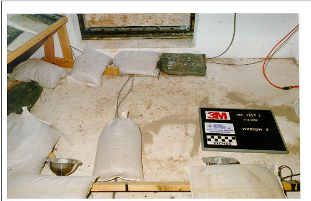
Figure A.80. Test 2. Posttest view of the glass debris on the South Structure floor (3M T2 POST 22.tif).
