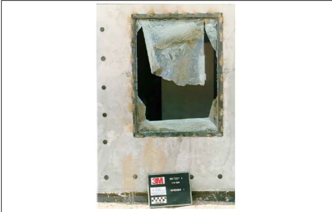
Figure A.99. Test 3. Posttest, exterior view of window 3 (3M T3 POST 11.tif).
