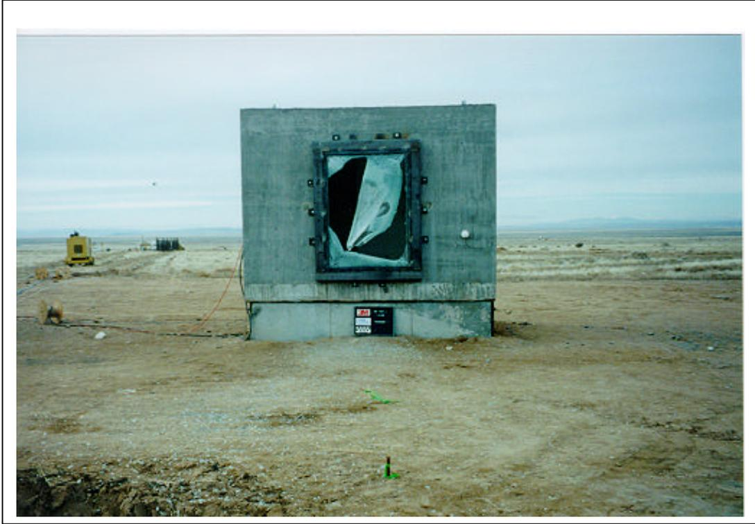
Figure A.54. Test 2. Posttest, exterior view of window 1 (3m sd T2 post28.tif).
