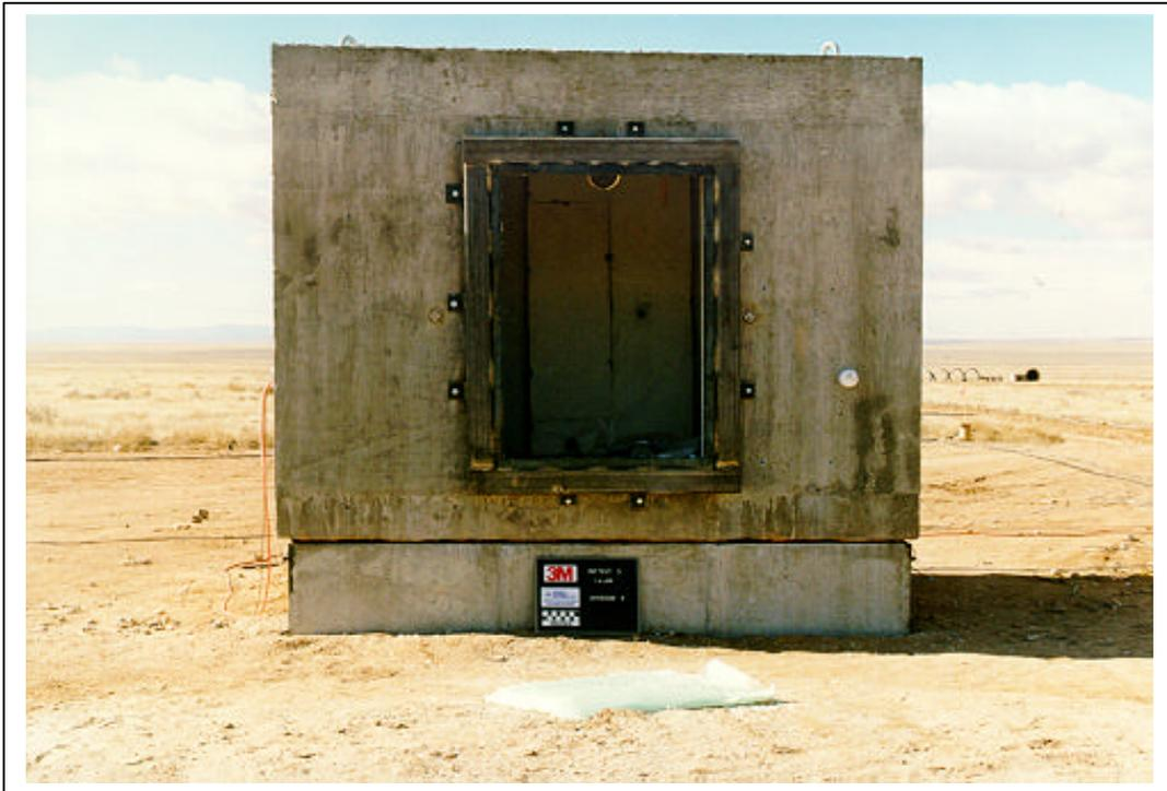
Figure A.174. Test 5. Posttest, exterior view of window 4 (3M T5 POST 37. tif).
