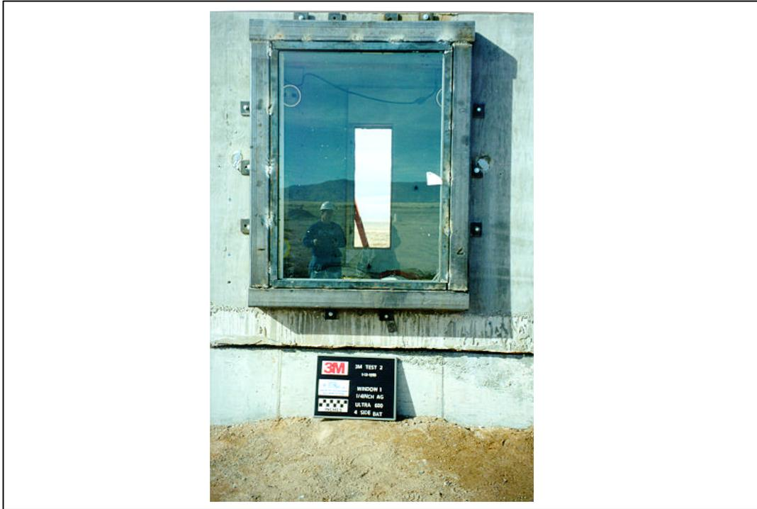
Figure A.52. Test 2. Pretest, exterior view of window 1 (3m sd T2 pre10.tif).
