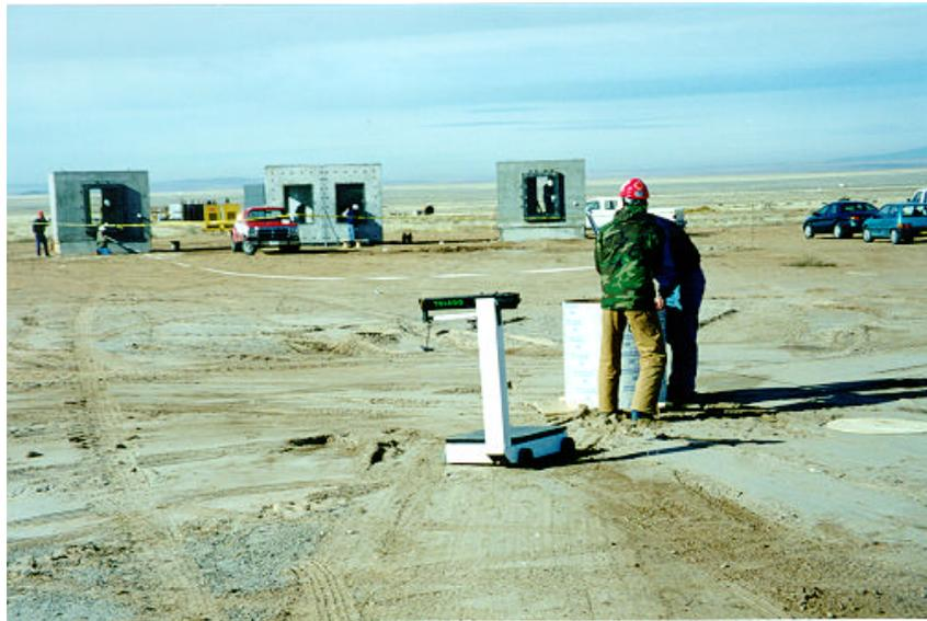
Figure 2.8. Technicians measuring charge standoff distance.
