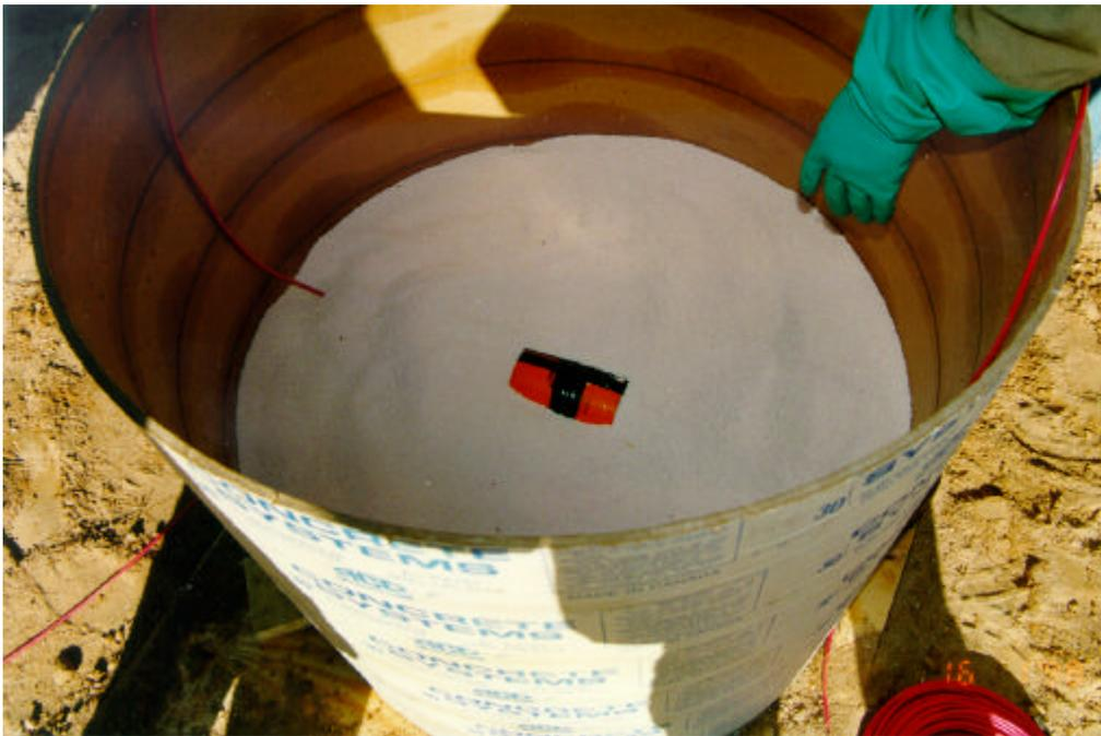
Figure 2.7. Pentolite booster in the center of the charge.
