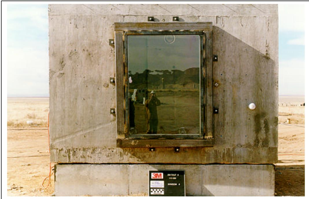
Figure A.139. Test 4. Pretest, exterior view of window 4 (3M T4 PRE 11.tif).
