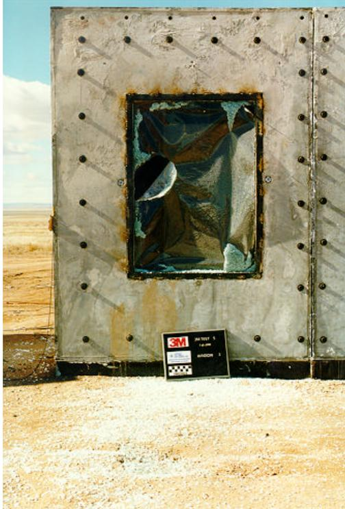
Figure 7.6. Exterior posttest view of window 3, test 5 (3M T5 post 32.tif).
