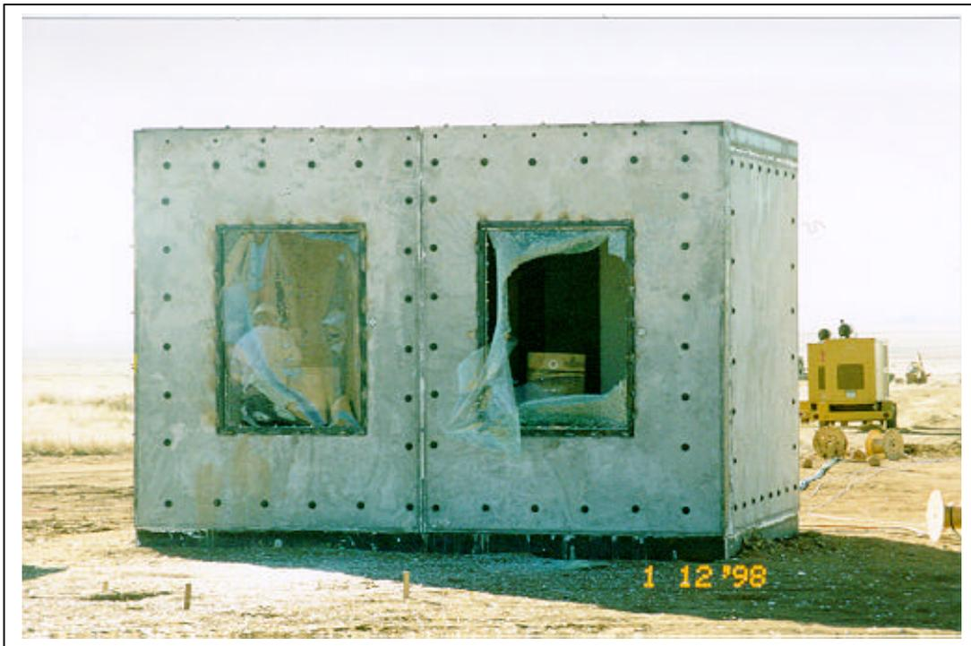
Figure A.27. Test 1. Posttest, exterior view of windows 2 and 3 (3M T1 F22.tif).
