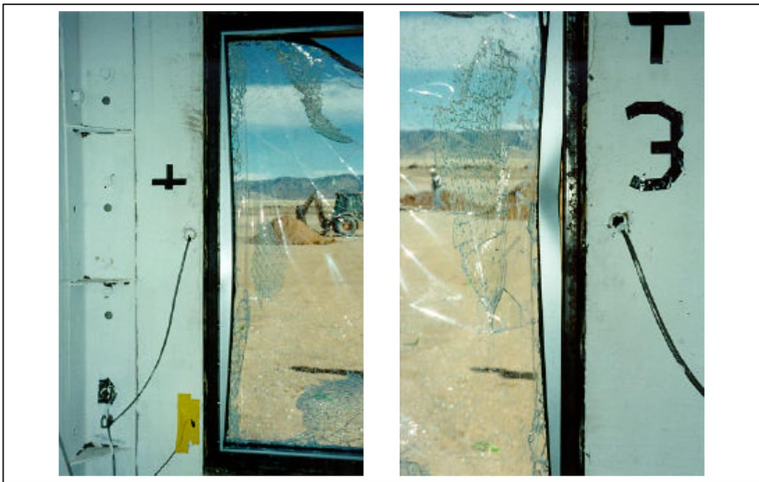
Figure A.138. Test 4. Posttest, interior views of window 3. Pictures of the aluminum frame displacement along the vertical edges (3m sd T4 post04.tif, 3m sd T4 post03.tif).
