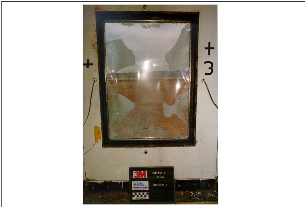
Figure A.199. Test 6. Posttest, interior view of window 3 (3M T6 POST 35.tif).
