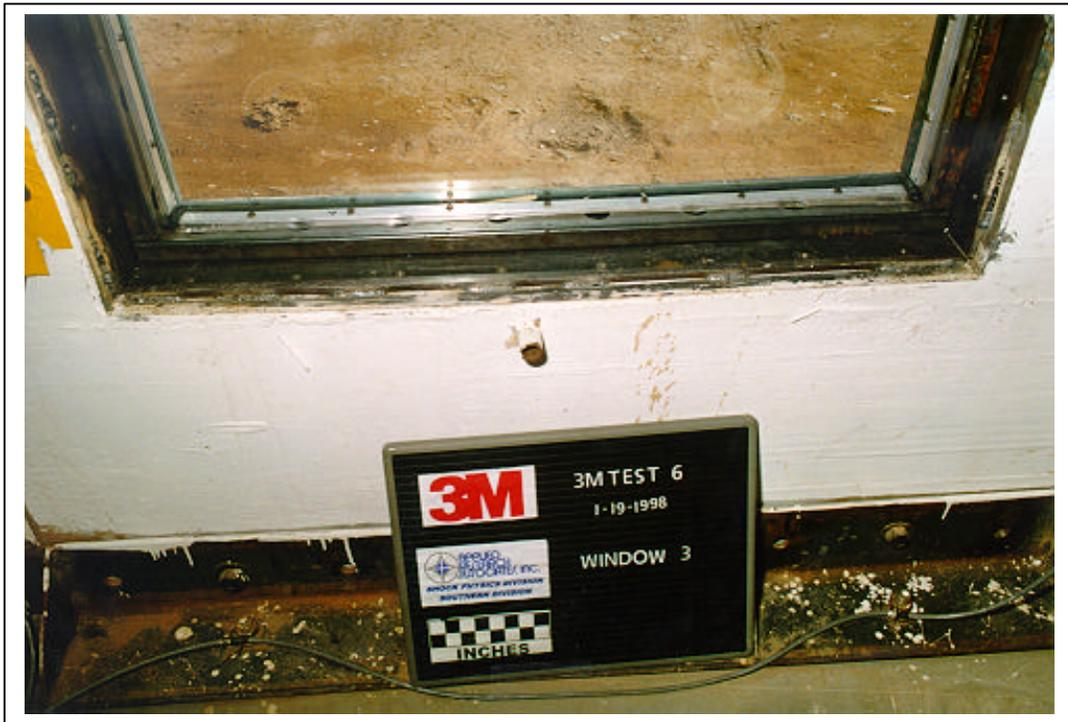
Figure A.197. Test 6. Pretest, interior view of window 3. Close-up view of the batten system (3M T6 PRE 09.tif).
