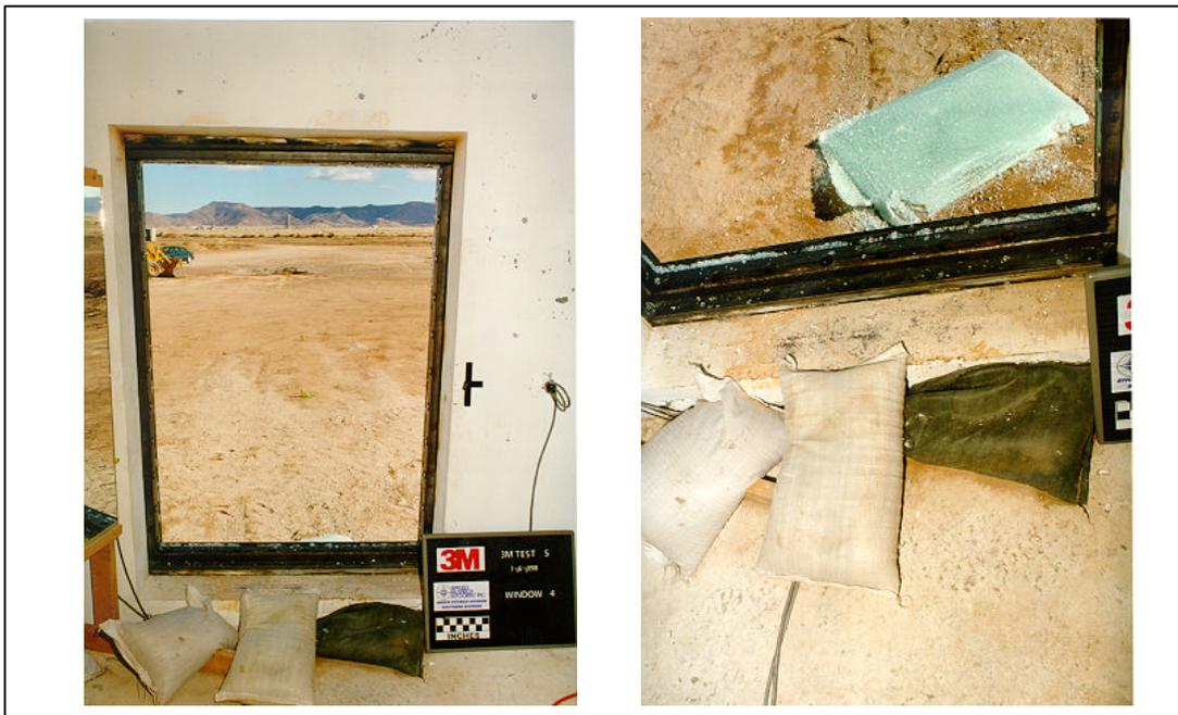
Figure A.176. Test 5. Posttest, interior views of window 4 (3M T5 POST 43.tif, 3M T5 POST 45.tif).
