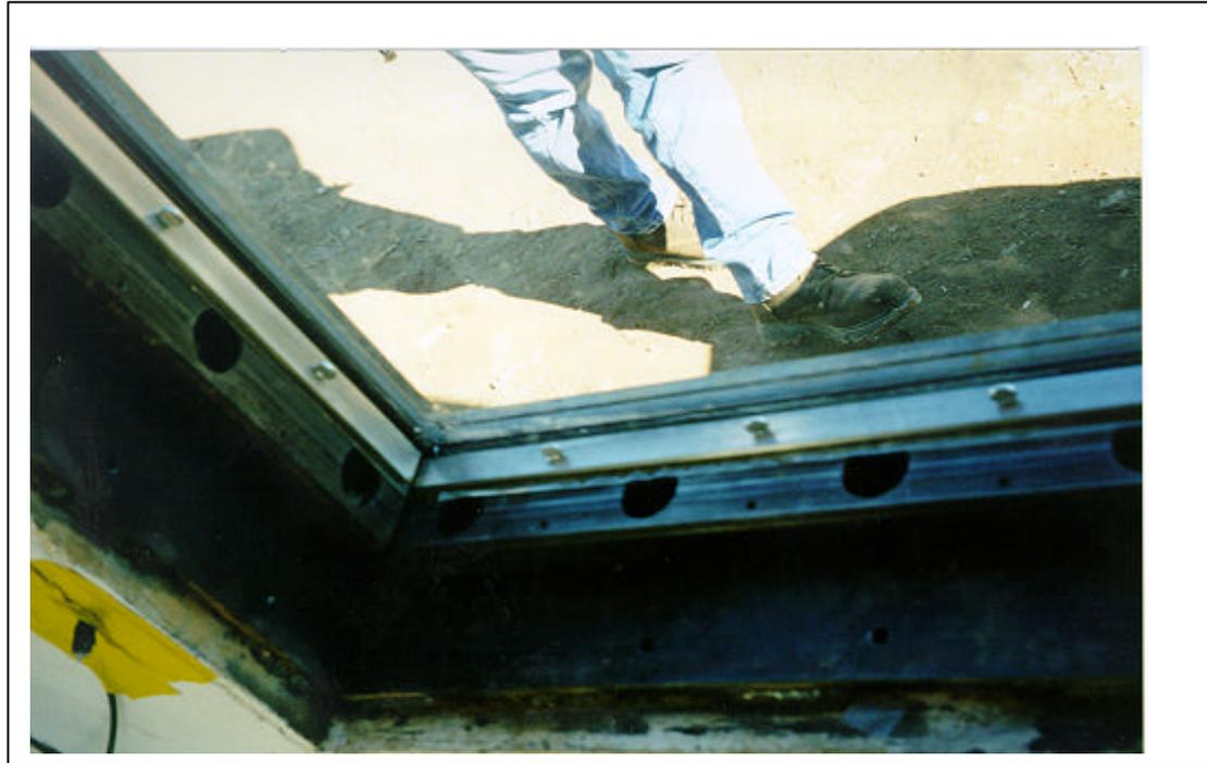
Figure A.33. Test 1. Pretest, interior view of window 3. Close up view of the batten system (3m sd T1 pre05.tif).
