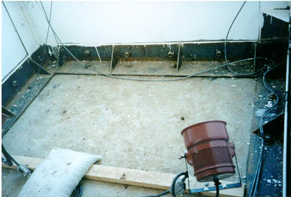
Figure 3.5. Interior view of glass fragmentation from window 2, test 1 (3M SD T1 post 18.tif).
