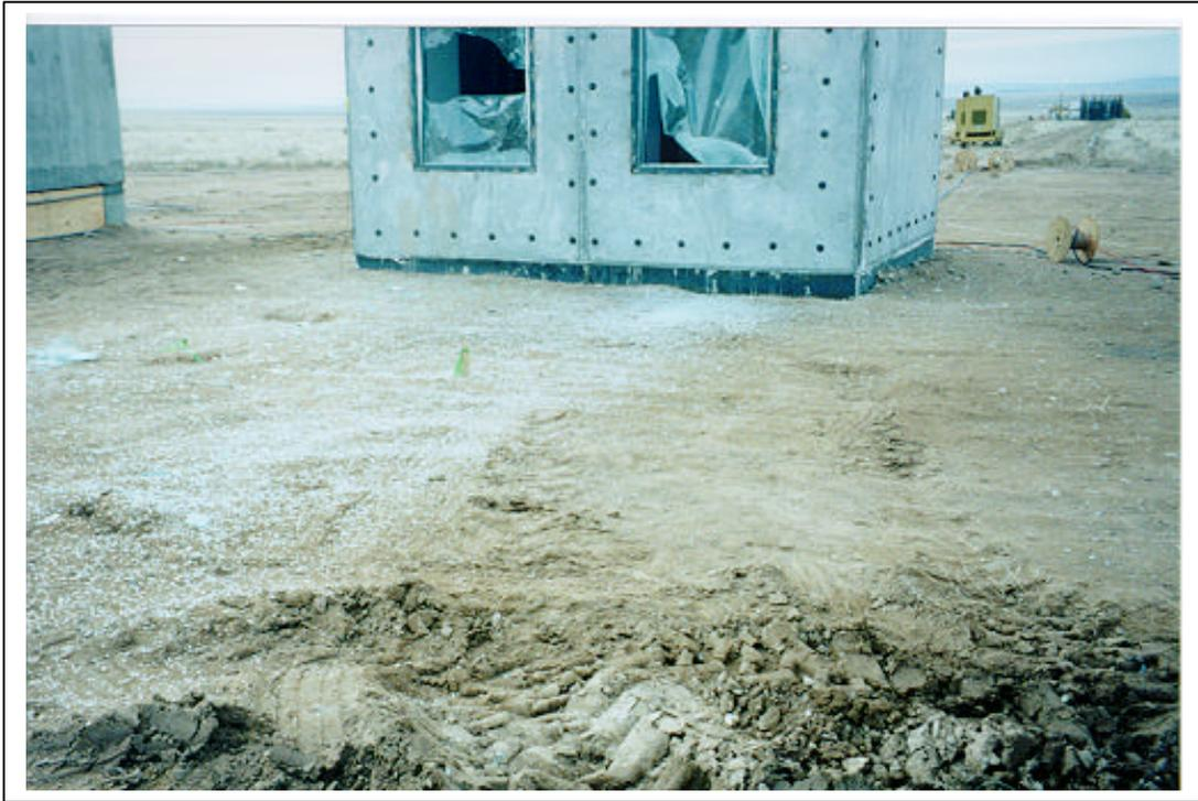
Figure A.64. Test 2. Posttest, exterior view of windows 2 and 3 (3m sd T2 post30 .jpg).
