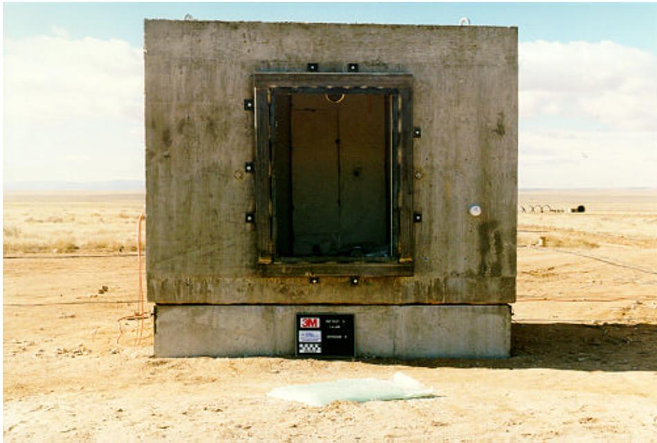
Figure 7.8. Exterior posttest view of window 4, test 5 (3M T5 post 37.tif).
