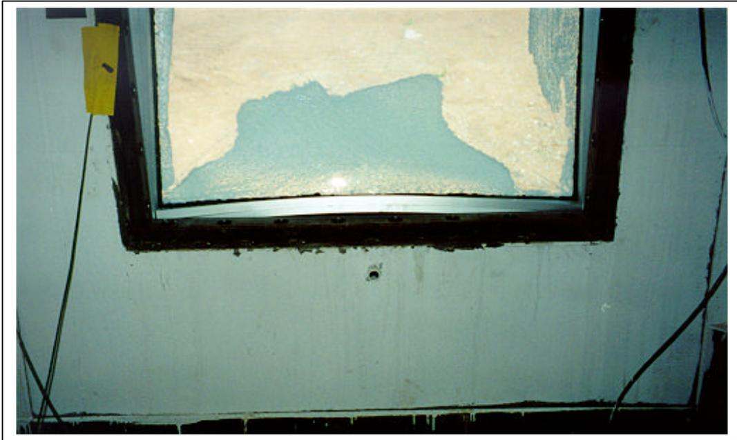
Figure A.132. Test 4. Posttest, interior view of window 2. Picture of the aluminum frame displacement along the bottom edge (3m sd T4 post02.tif).
