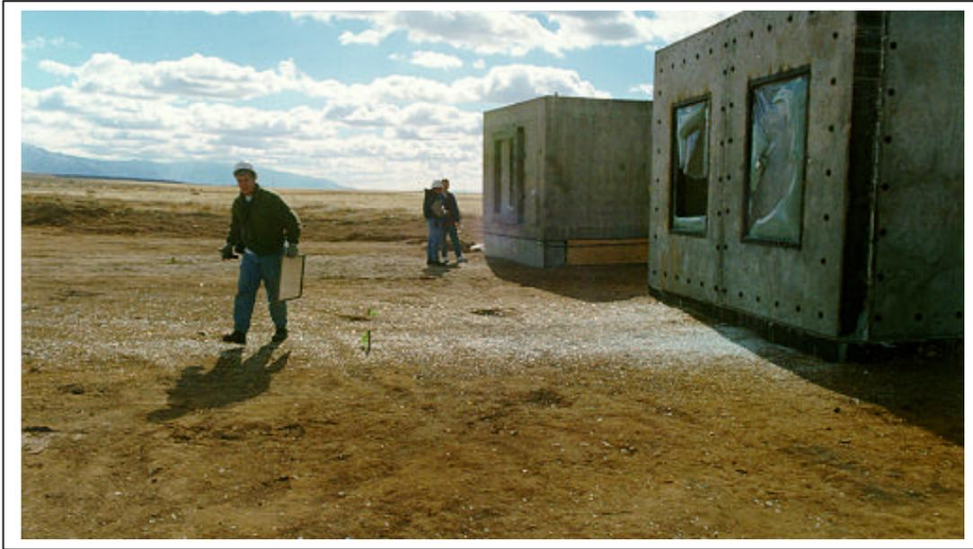
Figure A.103. Test 3. Posttest, exterior view of windows 2 and 3. Picture depicting the glass fragment spray in front of the reaction structures (3M T3 POST 20.tif).
