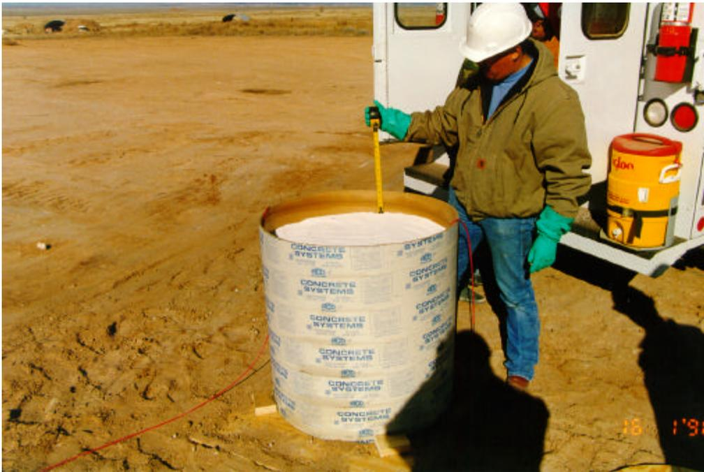
Figure 2.6. Test charge(diameter = 30 inches, height = 26.7 inches).
