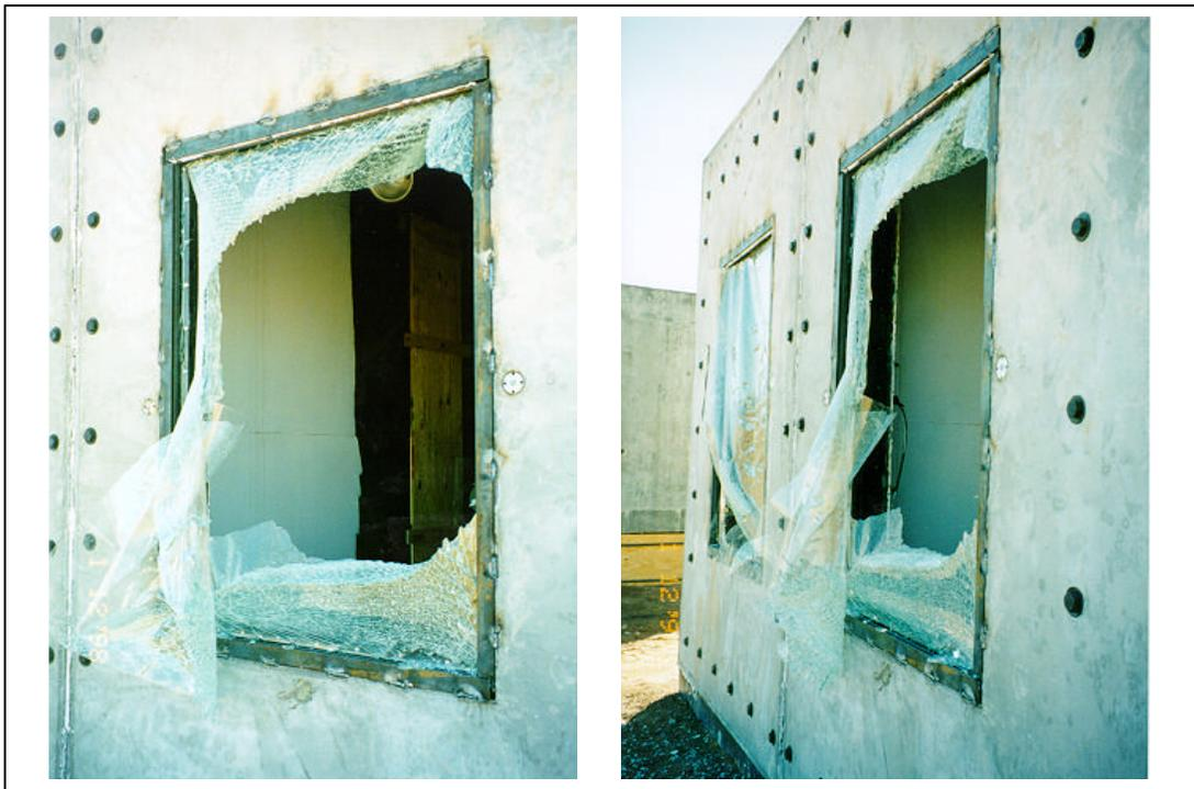
Figure A.29. Test 1. Posttest, exterior views of window 2 (3M T1 F17.tif, 3M T1 F18.tif ).
