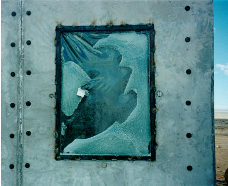
Figure 5.4. Exterior posttest view of window 2, test 3 (3M SD T3 post 19.tif).
