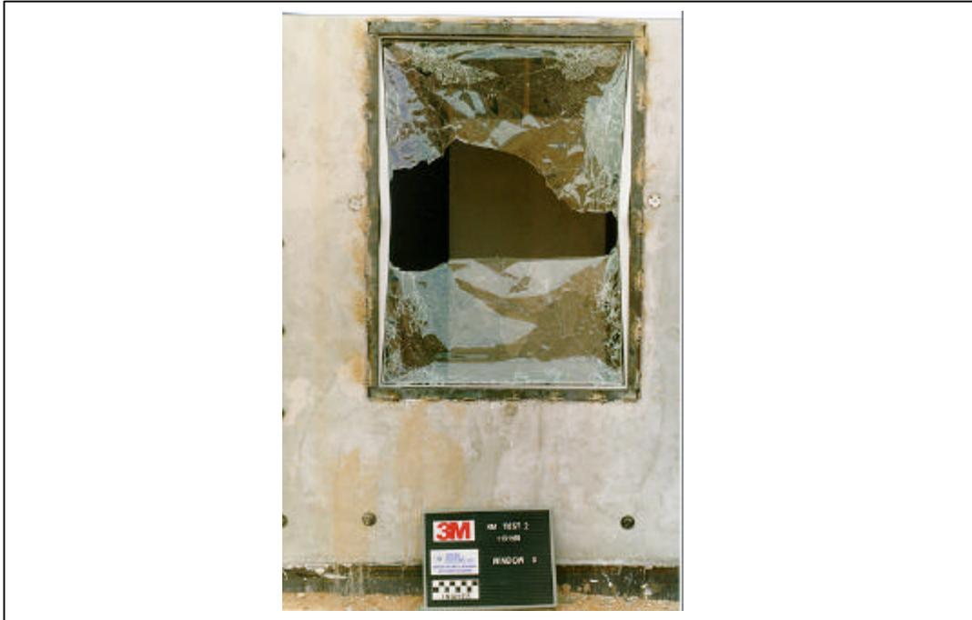
Figure A.68. Test 2. Posttest, exterior view of window 3 (3M T2 POST 15.tif).
