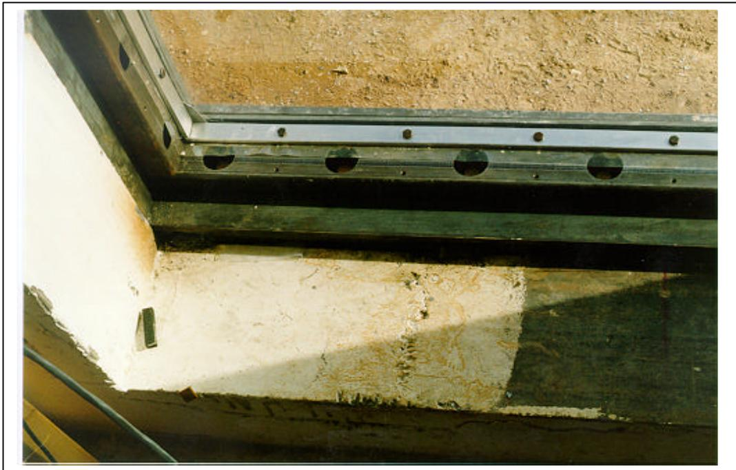
Figure A.61 Test 2. Pretest, interior view of window 2. Close-up view of the batten system (3M T2 PRE 09.tif).
