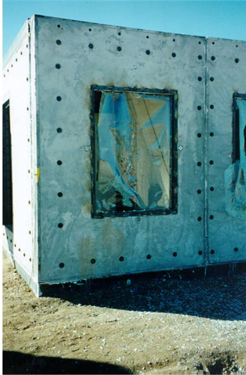
Figure 3.6. Exterior posttest view of window 3, test 1 (3M SD T1 post 36.tif).
