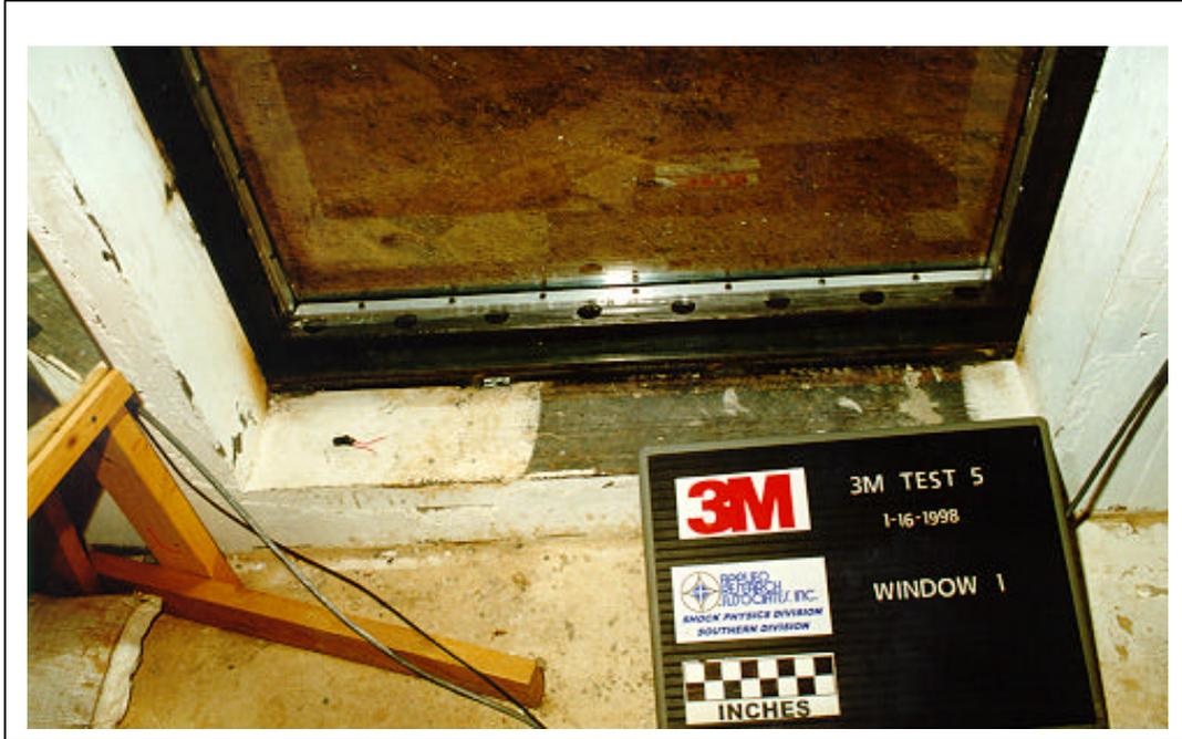
Figure A.151. Test 5. Pretest, interior view of Window 1. Close-up view of the batten system (3M T5 PRE 07.tif).
