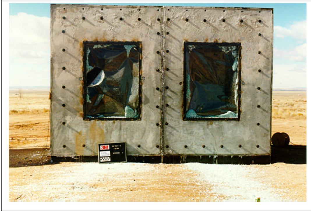
Figure A.159. Test 5. Posttest, exterior view of windows 2 and 3 (3M T5 POST 33.tif).
