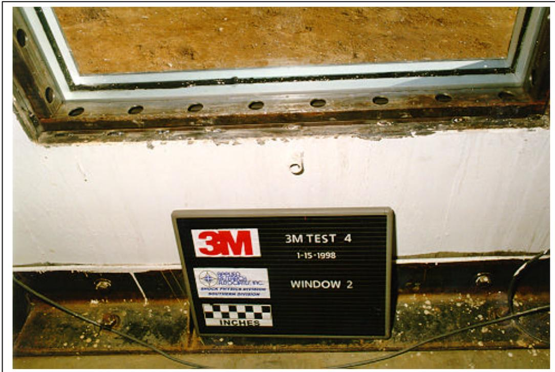
Figure A.126. Test 4, pretest interior view of window 2. Picture showing wet glazed application (3M T4 PRE 05.tif).
