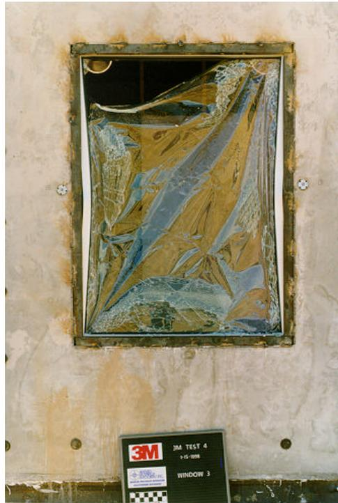
Figure 6.5. Exterior posttest view of window 3, test 4 (3M T4 post 12.tif).
