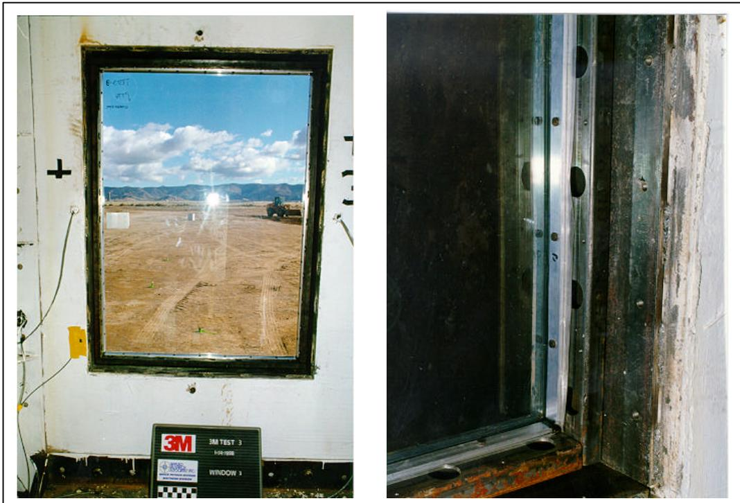
Figure A.98. Test 3. Pretest, interior views of window 3. Close-up view of the batten system shown on right (3M T3 PRE 07.tif, 3M T3 PRE 08.tif).
