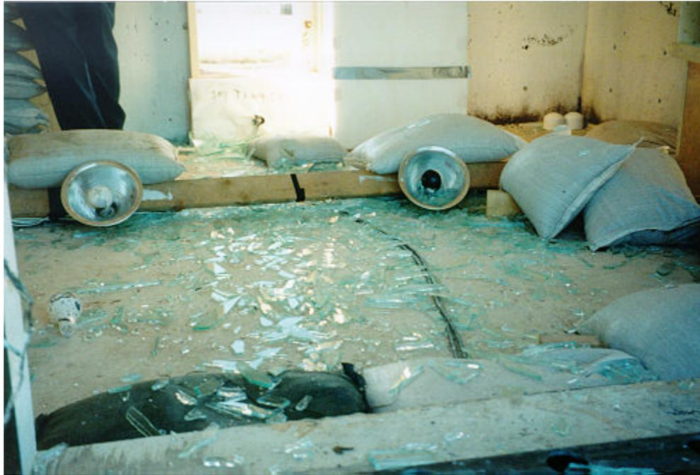
Figure 3.9. Interior view of glass fragmentation from window 4, test 1 (3M SD T1 post 16.tif).
