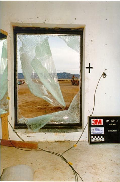
Figure 4.3. Interior view of window 1 and fragmentation, test 2 (3M T2 post 19.tif).
