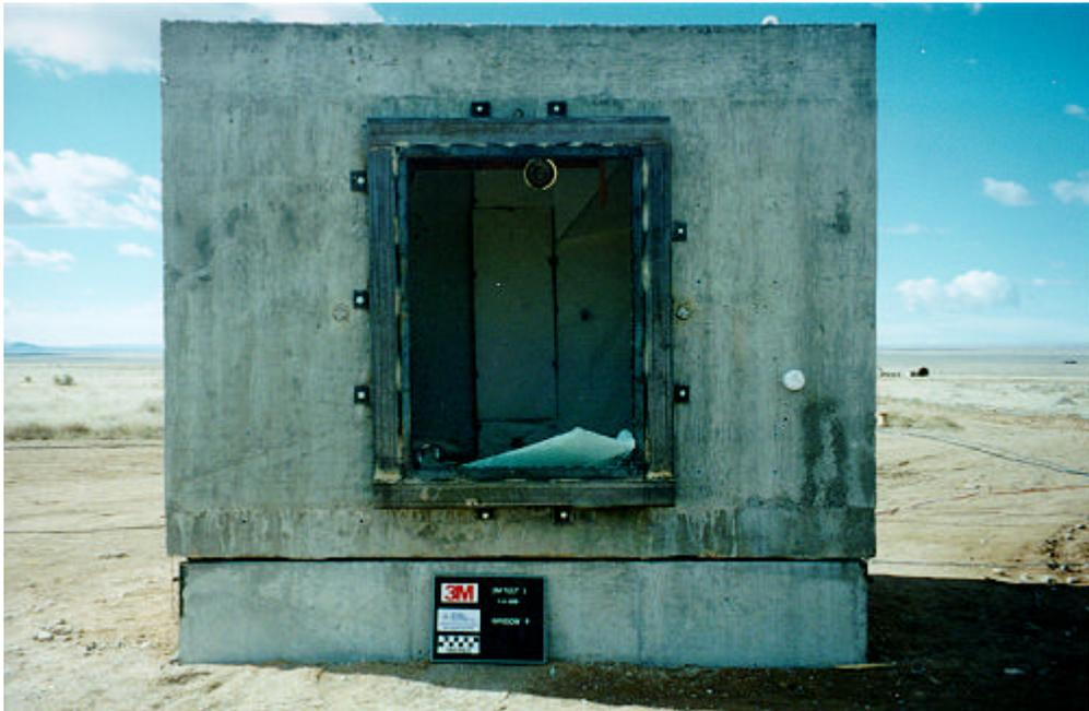
Figure 5.7. Exterior posttest view of window 4, test 3 (3M SD T3 post 14.tif).
