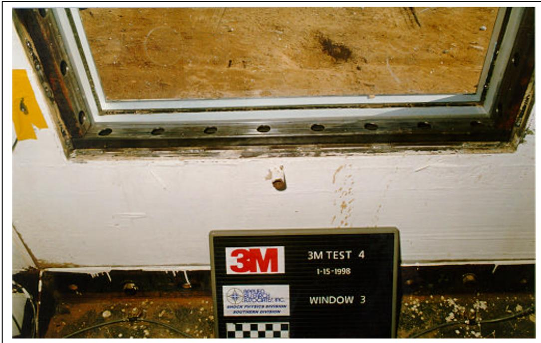
Figure A.135. Test 4. Pretest, interior view of window 3. Close-up view of the batten system (3M T4 PRE 07.tif).
