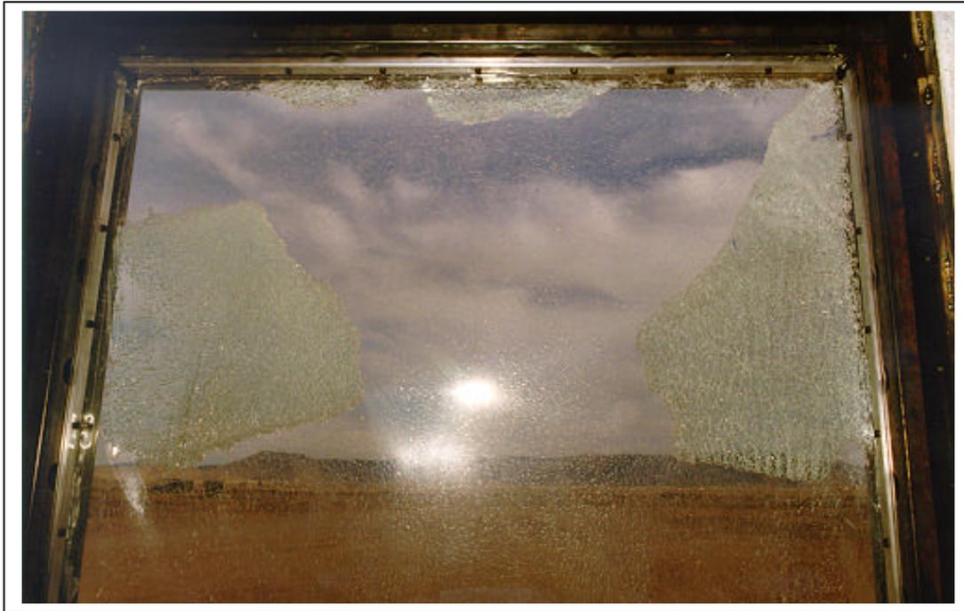
Figure A.201. Test 6. Posttest, interior view of window 3 (view of top half)
