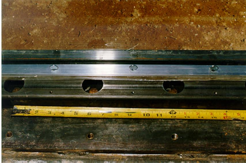
Figure 3.2. Thumb-screw attachment of batten for test 1, windows 2 and 3 (3M T1 pre 01.tif).
