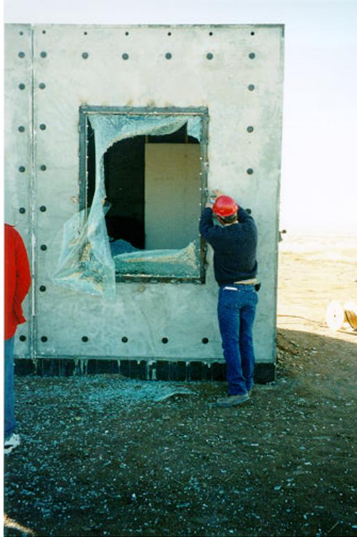
Figure 3.4. Exterior posttest view of window 2, test 1(3M SD T1 post 20.tif).
