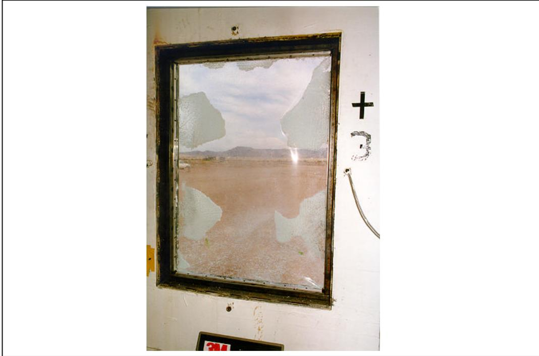
Figure A.200. Test 6. Posttest, interior view of window 3 (3M T6 POST 36.tif).
