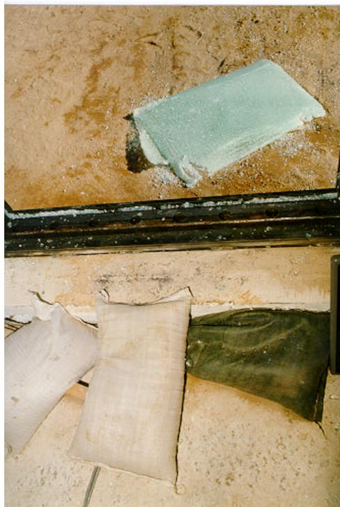
Figure 7.9. Interior view of window 4 fragmentation, test 5 (3M T5 post 47.tif).
