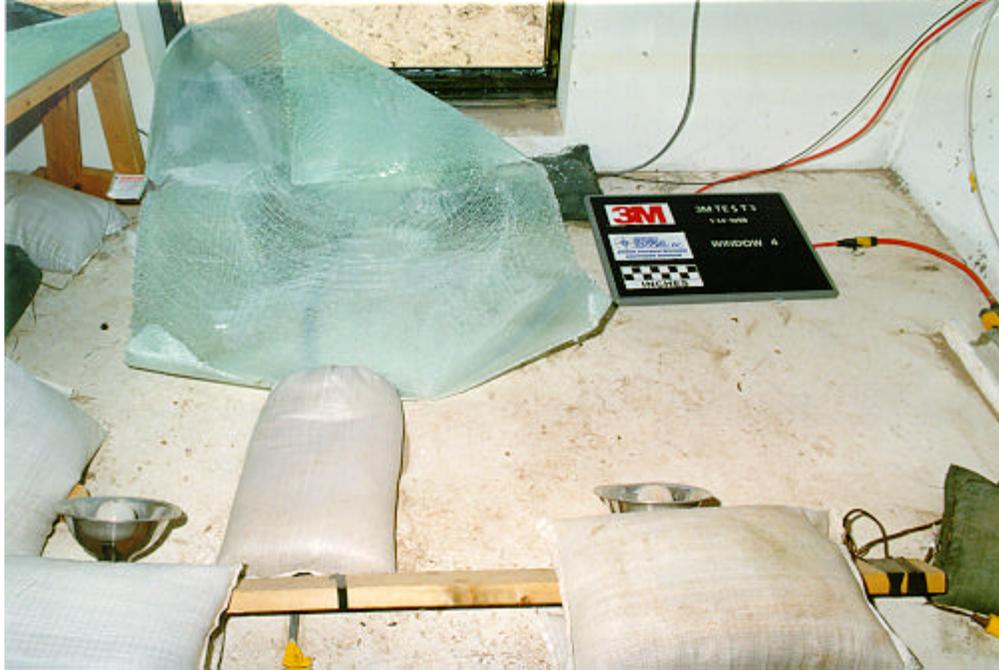
Figure 5.8. Interior view of window 4 and fragmentation, test 3 (3M T3 post 01.tif).
