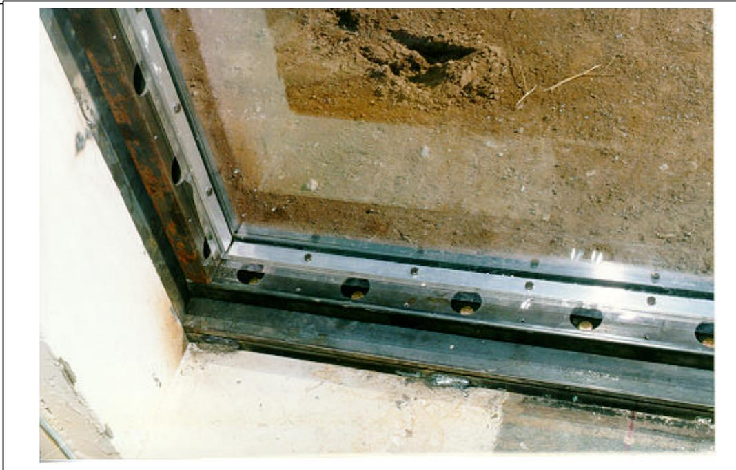
Figure A.85. Test 3. Pretest interior view of window 1. Close-up view of the batten system (3M T3 PRE 02.tif).
