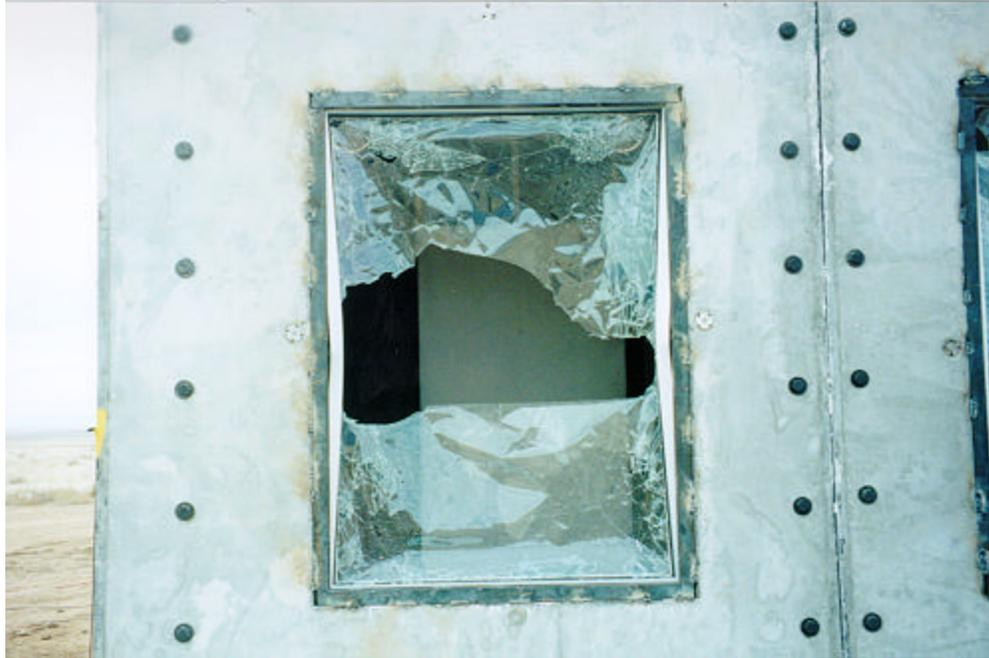
Figure 4.6. Exterior posttest view of window 3, test 2 (3M SD T2 post 37.tif).
