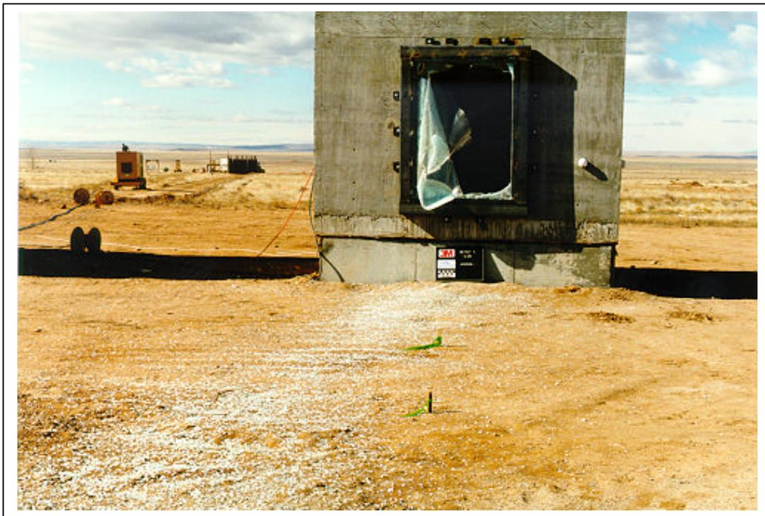
Figure A.152. Test 5. Posttest, exterior view of window 1 (3M T5 POST 24. tif).
