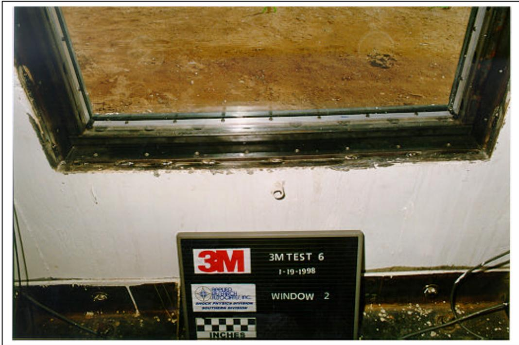
Figure A.191. Test 6. Pretest interior view of window 2. Close-up view of the batten system (3M T6 PRE 07.tif).
