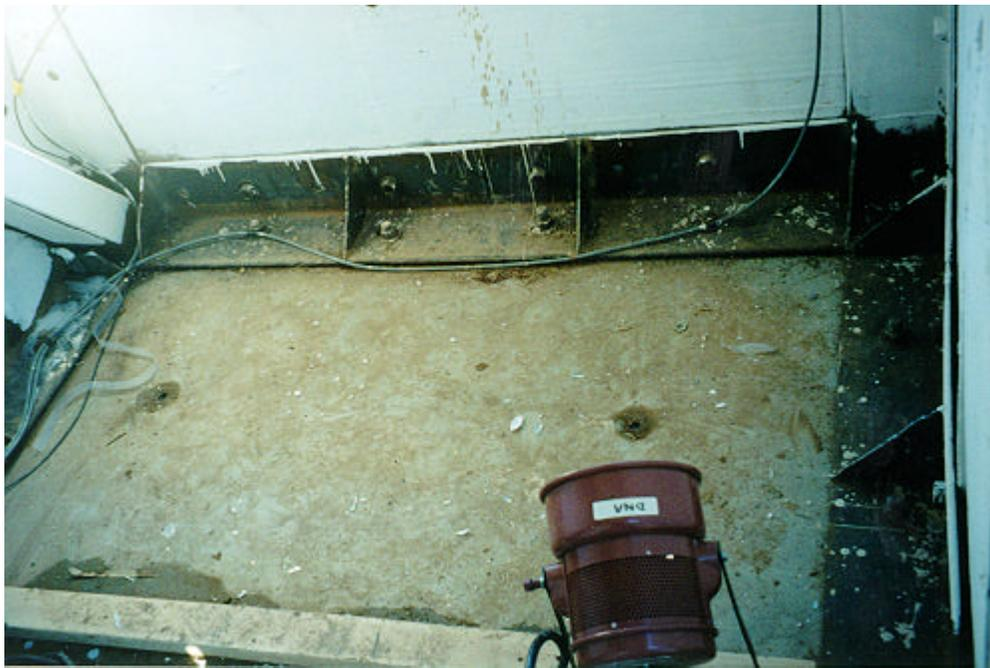
Figure 3.7. Interior view of glass fragmentation from window 3, test 1 (3M SD T1 post 31.tif).
