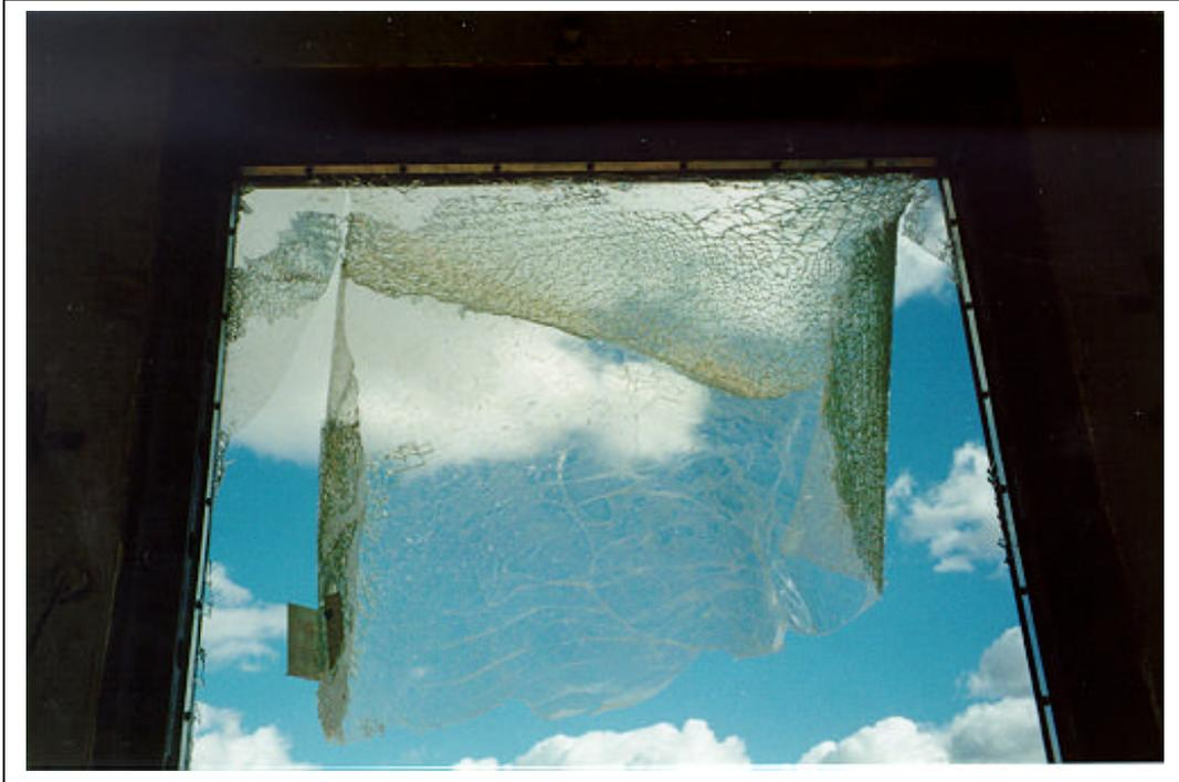
Figure A.101. Test 3. Posttest, interior view of window 3 (top half)
