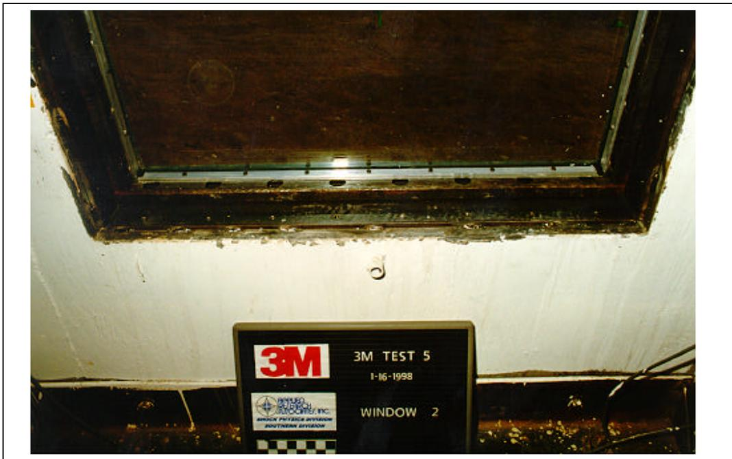
Figure A.158. Test 5. Pretest, interior view of window 2. Close-up view of the batten system (3M T5 PRE 03.tif).
