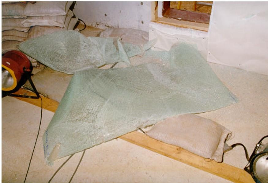
Figure 8.3. Interior posttest view of window 1 fragmentation near the rear of the structure, test 6 (3M T6 post 21.tif).
