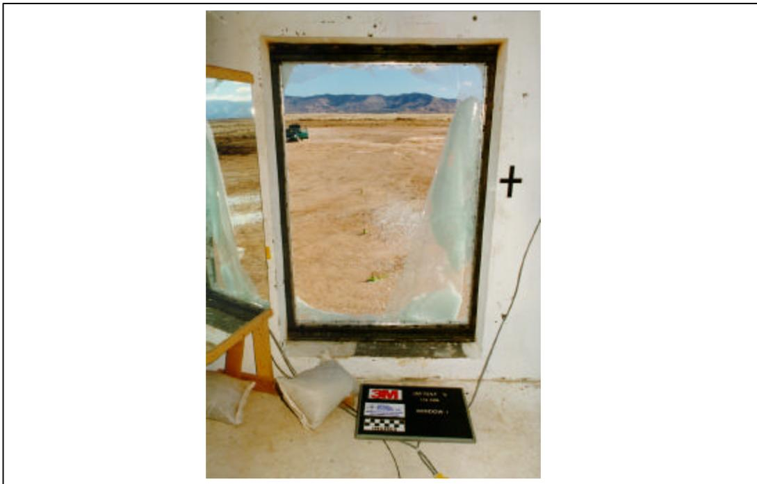
Figure A.154. Test 5. Posttest, interior view of window 1 (3M T5 POST 06.tif).
