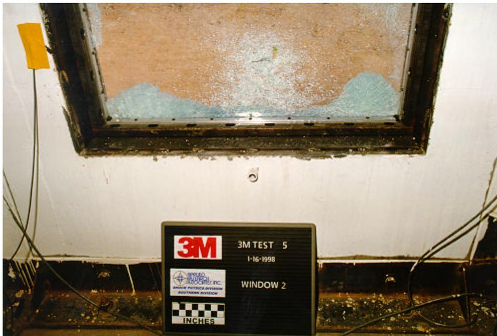
Figure 7.5. Interior view of window 2 frame deformation, test 5 (3M T5 post 06.tif).
