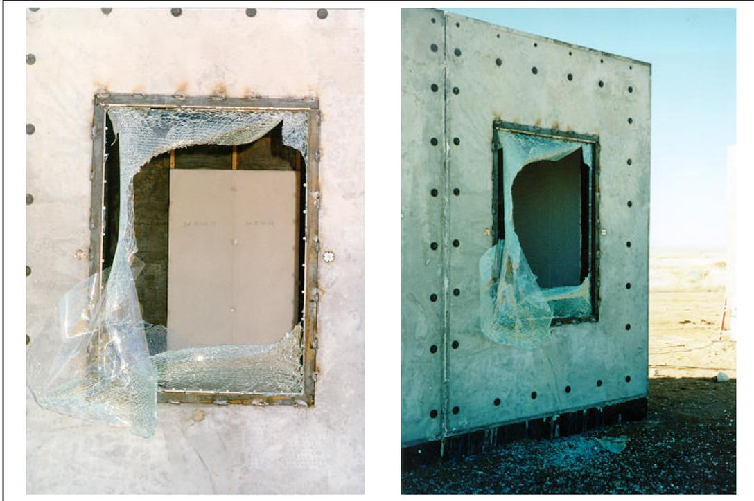
Figure A.28. Test 1. Posttest, exterior views of window 2 (3M T1 POST 07.tif, 3m sd t1 post25.tif).
