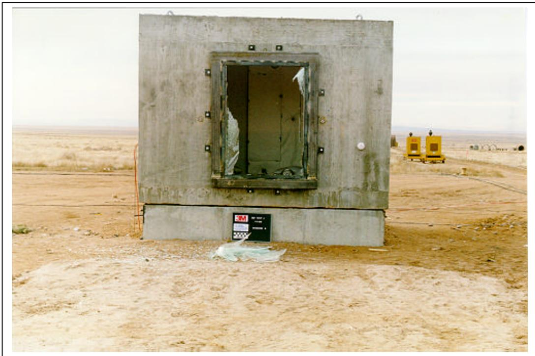
Figure A.77. Test 2. Posttest, exterior view of window 4 (3M T2 POST 02.tif).
