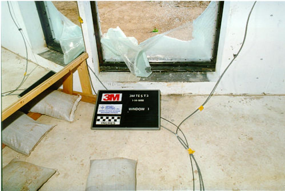
Figure 5.3. Interior view of window 1 and fragmentation, test 3 (3M T3 post 23.tif).
