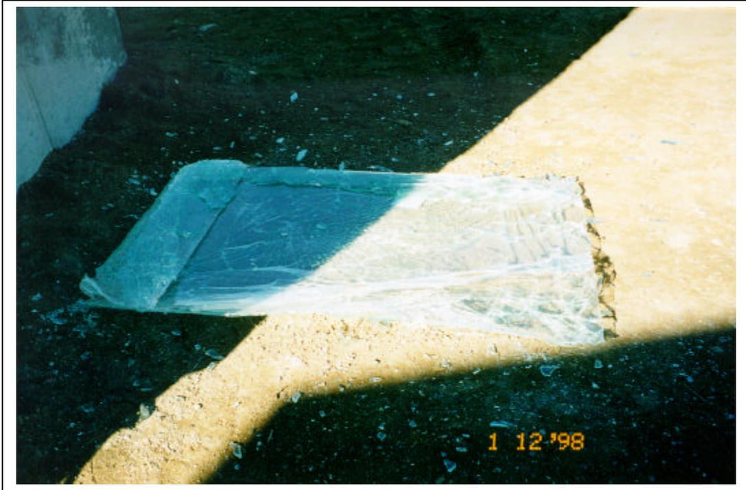
Figure A.20. Test 1. Posttest view of the security film and attached glazing from window 1 (3M T1 F51.tif).
