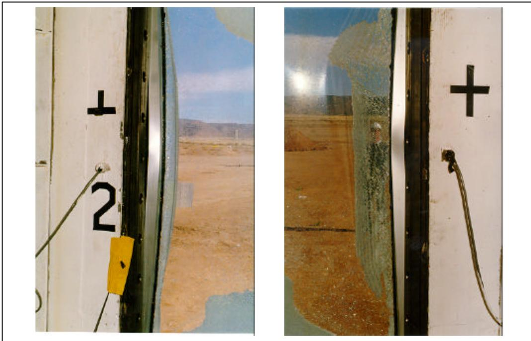
Figure A.130. Test 4. Posttest, interior views of window 2. Pictures of the aluminum frame displacement along the vertical edges (3M T4 POST 16.tif).
