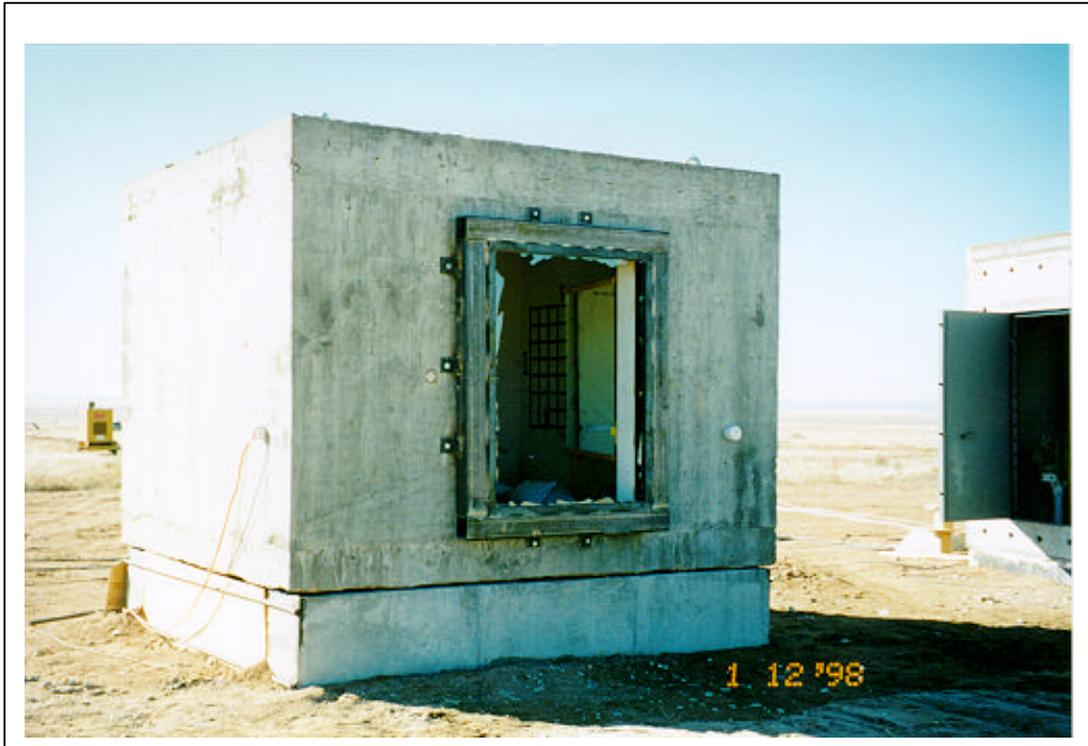
Figure A.42. Test 1. Posttest, exterior view of window 4 (3M T1 F61.tif).
