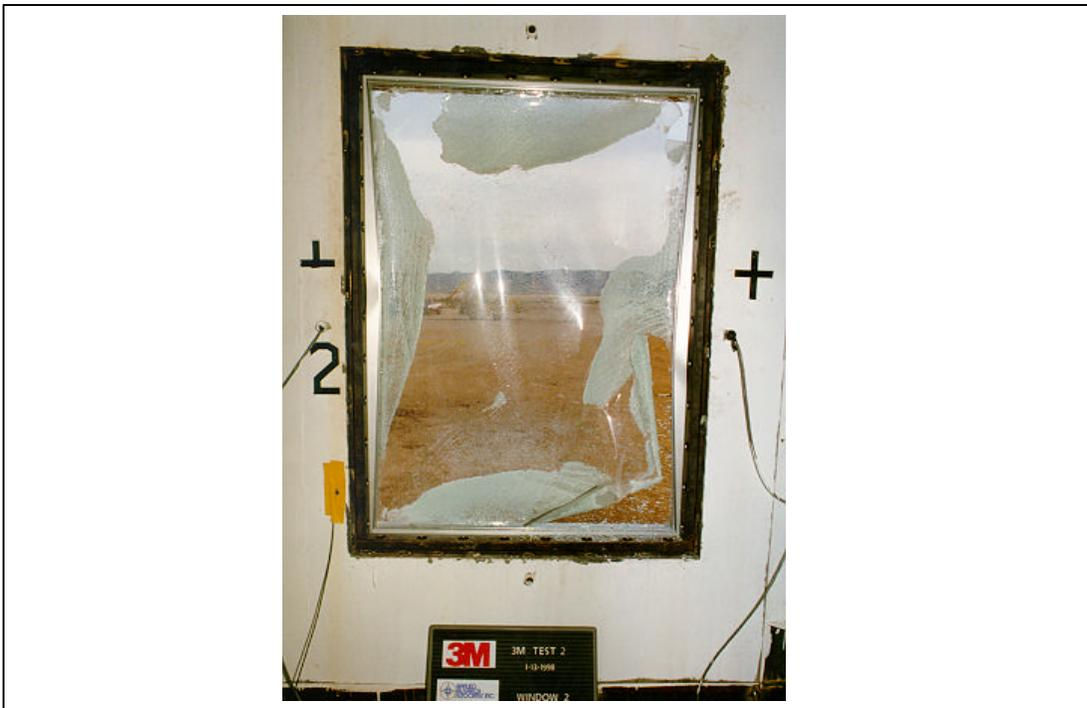
Figure A.65. Test 2. Posttest, interior view of window 2 (3M T2 POST 23.tif).
