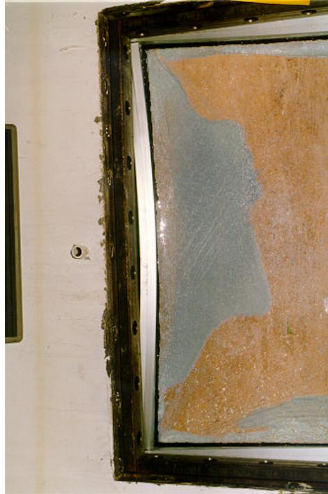
Figure 6.4. Interior view of window 2 frame deformation, test 4 (3M T4 post 14.tif).
