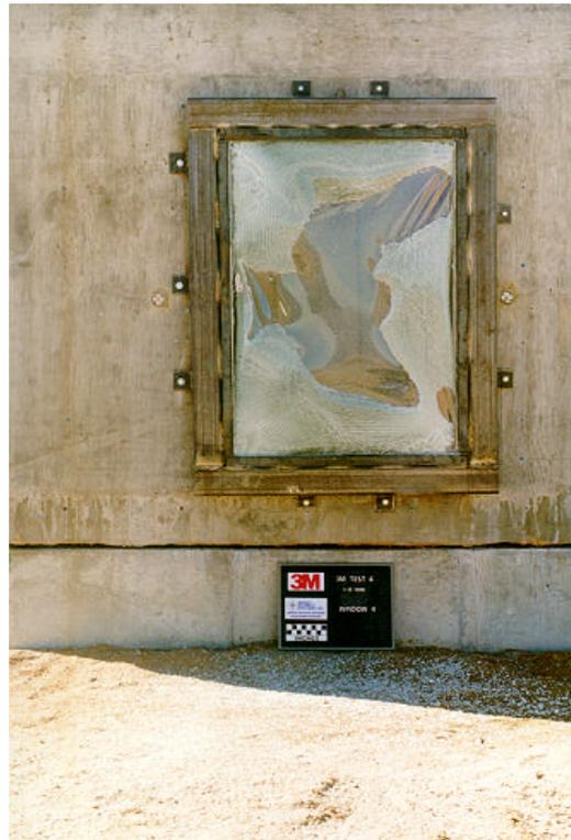
Figure 6.7. Exterior posttest view of window 4, test 4 (3M T4 post 44.tif).
