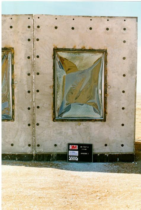
Figure 6.3. Exterior posttest view of window 2, test 4 (3M T4 post 10.tif).
