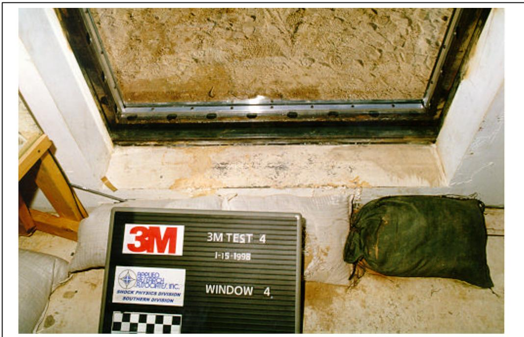
Figure A.142. Test 4. Pretest, interior view of window 4. Close-up view of batten system (3M T4 PRE 09.tif).
