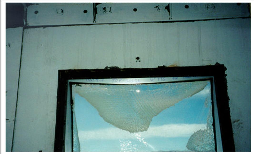
Figure A.131. Test 4. Posttest, interior view of window 2. Picture of the aluminum frame displacement along the top edge (3m sd T4 post02.tif).
