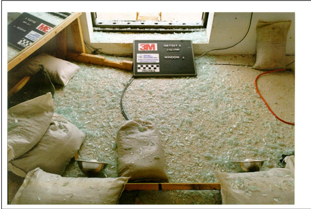
Figure A.212. Test 6. Posttest view of the South Structure floor (3M T6 POST 26.tif).
