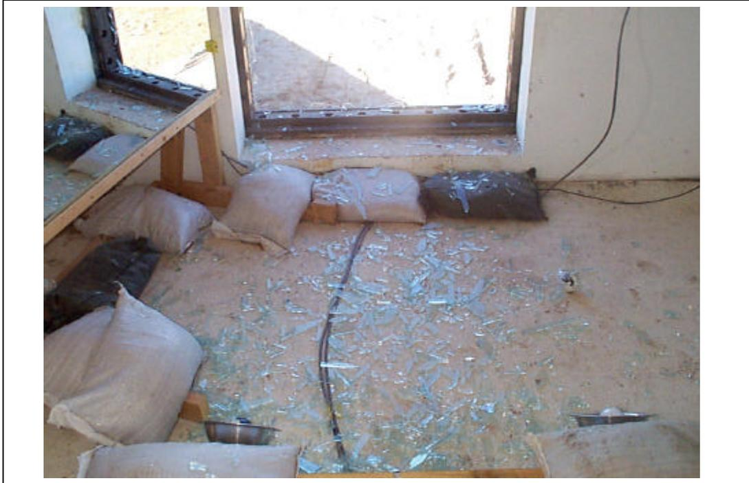
Figure A.45. Test 1. Posttest view of glass debris on the South Structure floor (test1\_42.jpg).
