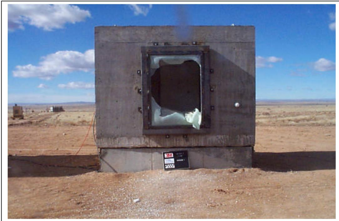
Figure A.86. Test 3. Posttest, exterior view of window 1 (test3\_22.jpg).
