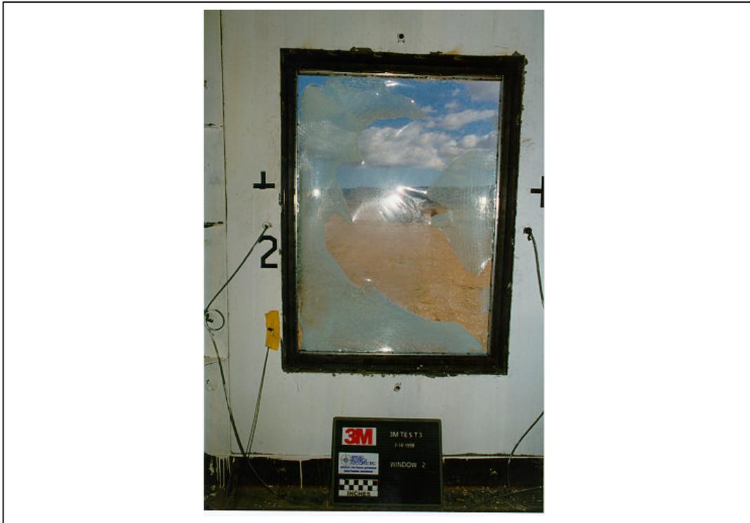
Figure A.95. Test 3. Posttest, interior view of window 2 (3M T3 POST 25.tif).
