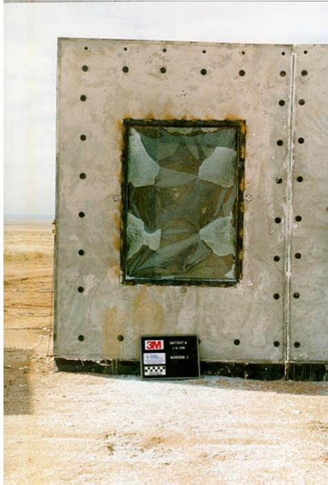
Figure 8.6. Exterior posttest view of window 3, test 6 (3M T6 post 04.tif).
