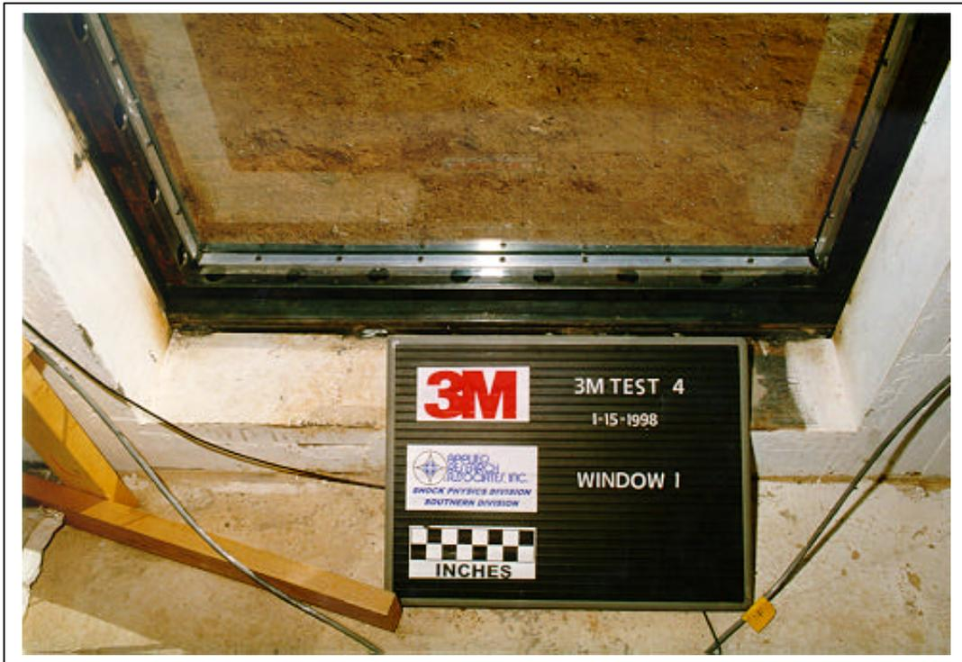
Figure A.118. Test 4. Pretest, interior view of window 1. Close-up view of the batten system (3M T4 PRE 02.tif).
