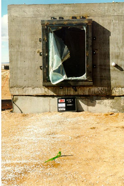
Figure 7.2. Exterior posttest view of window 1, test 5 (3M T5 post 25.tif).
