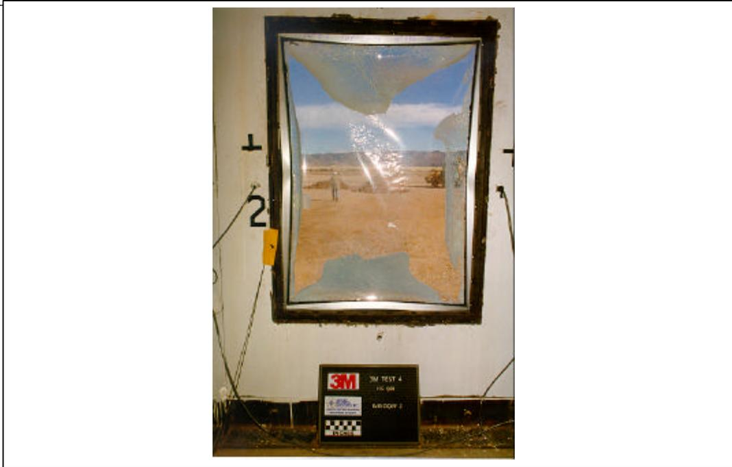
Figure A.129. Test 4. Posttest, interior view of window 2 (3M T4 POST 13.tif).
