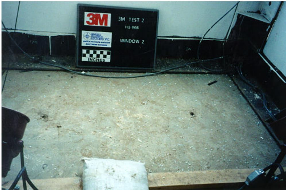
Figure 4.5. Interior view of glass fragmentation from window 2, test 2 (3M SD T2 post 12.tif).
