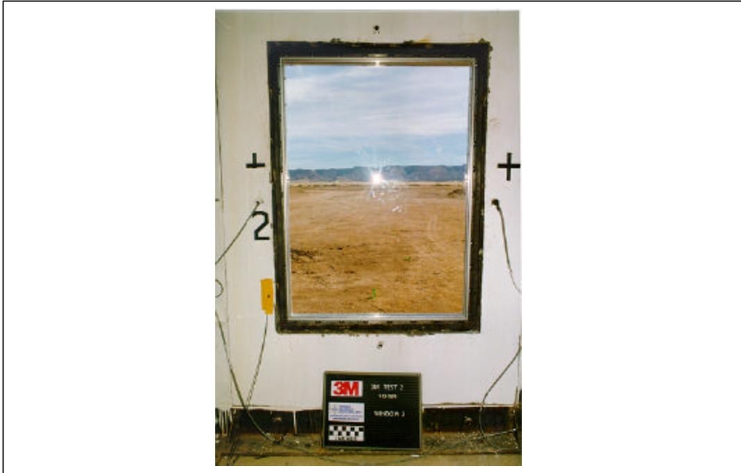
Figure A.60. Test 2. Pretest, interior view of window 2 (3M T2 PRE 08.tif).
