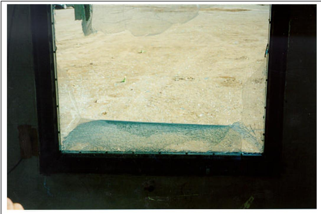
Figure A.102. Test 3. Posttest, interior view of window 3 (bottom half)
