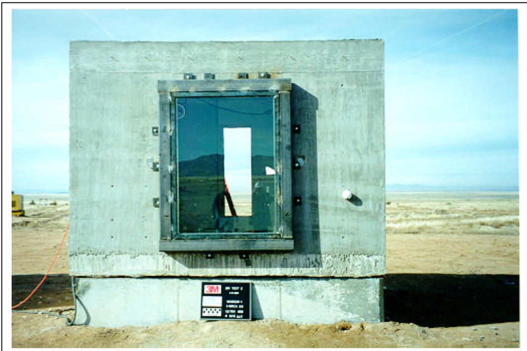
Figure A.51. Test 2. Pretest, exterior view of window 1 (3m sd T2 pre11.tif).
