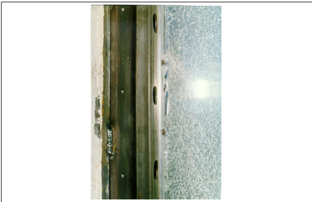
Figure A.96. Test 3. Posttest, interior view of window 2. Close-up view of a tear in the security film along the vertical edge (3M T3 POST 27.tif).
