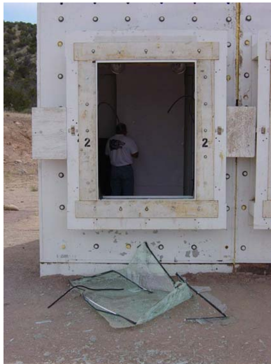
Figure 3-45 Exterior post-test view of window 2. (DSC04364.jpg)
