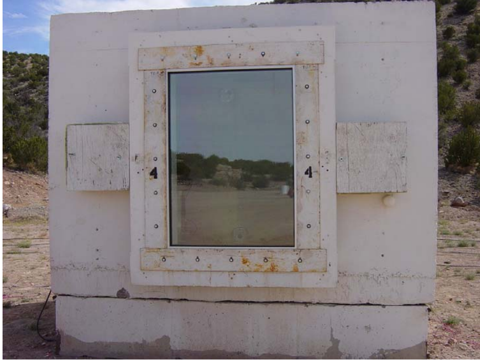
Figure 3-24 Exterior pre-test view of window 4. (DSC04141.jpg)
