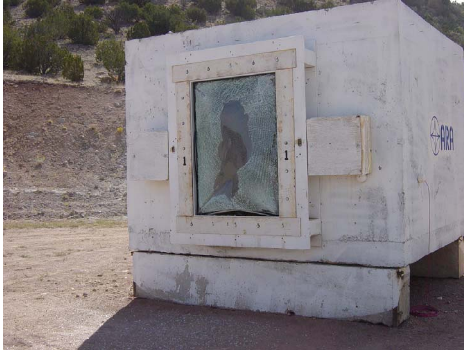
Figure 3-29 Exterior post-test view of window 1. (DSC4280.jpg)
