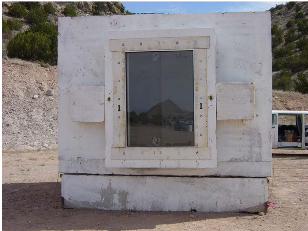
Figure 3-15 Exterior pre-test view of window 1. (DSC04110.jpg)
