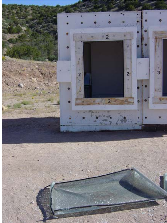
Figure 3.7. Exterior post-test view of Window 2.
