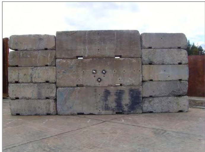
Figure 10: Reflected Pressure Transducers on gauge block
