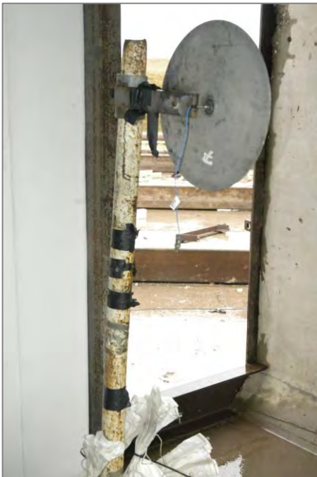
Figure 9: Free Field pressure transducer in aerodynamic housing
