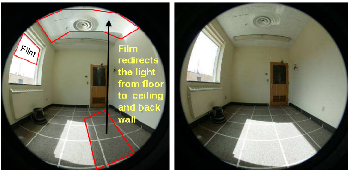
Figure 1. Photographs taken with a fisheye lens demonstrates the effectiveness of the daylight redirecting film.
