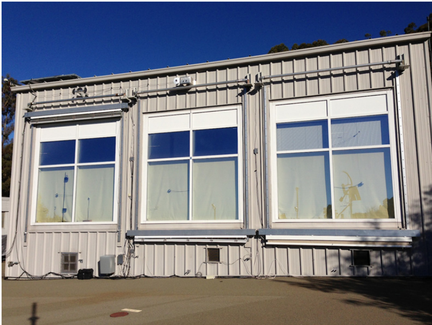
Fig. 1. Outdoor view of the LBNL windows testbed facility (Room A is on the right, B is in the center, and C is on the left).
