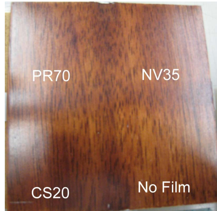
Red Oak Surface Before vs. After Exposure to UV
