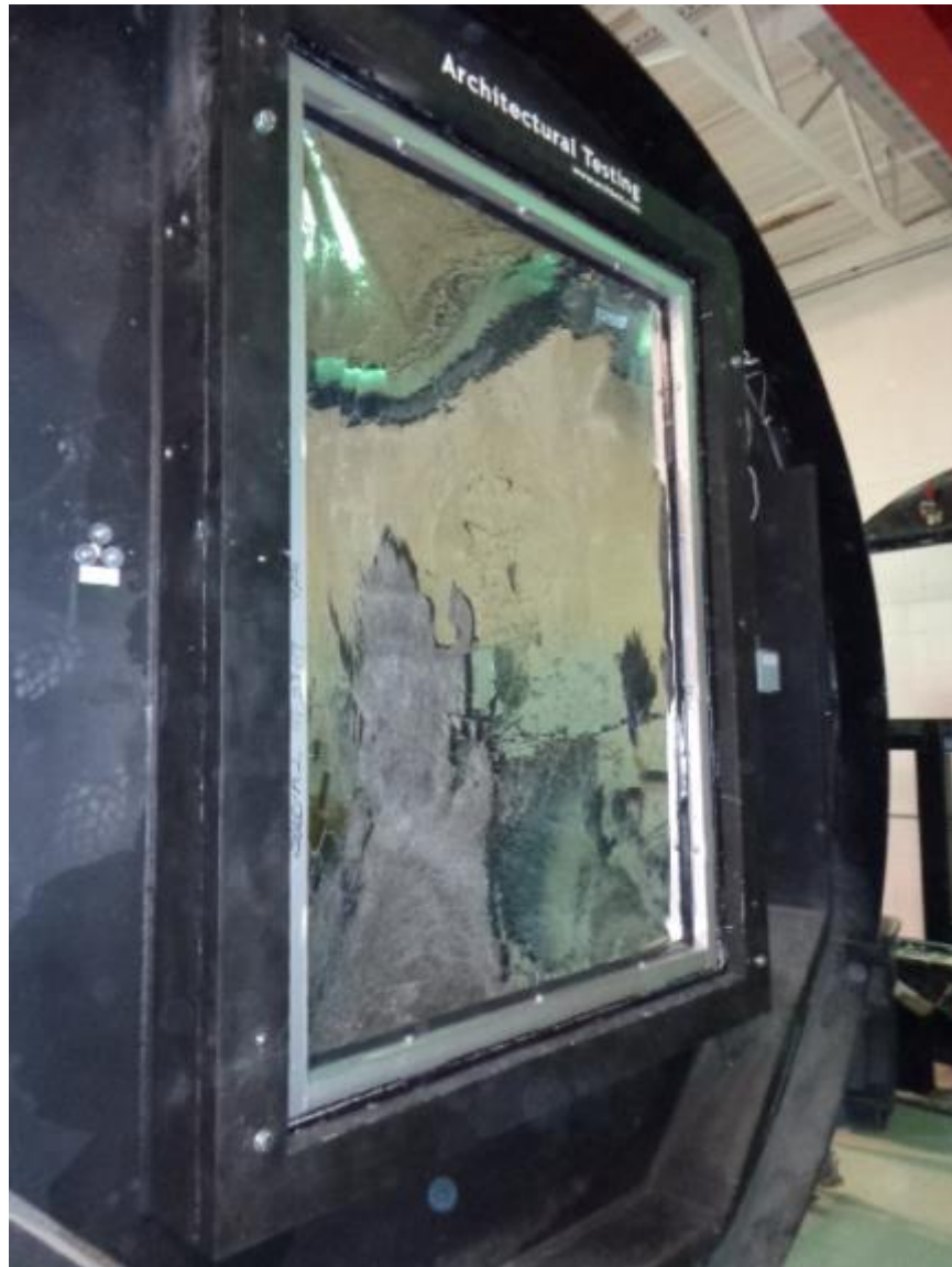
Photo No. 5 Post-test Specimen #2, Interior
