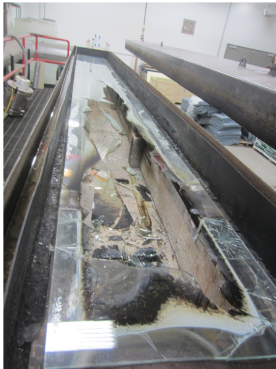
Photo No. 2 Unexposed Surface (Post-test) www.archtest.com
