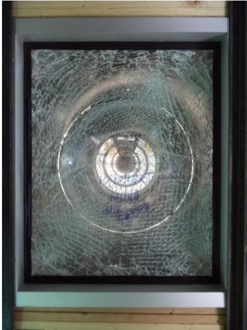
Photo No. 5 Post-test Specimen #2, Interior
