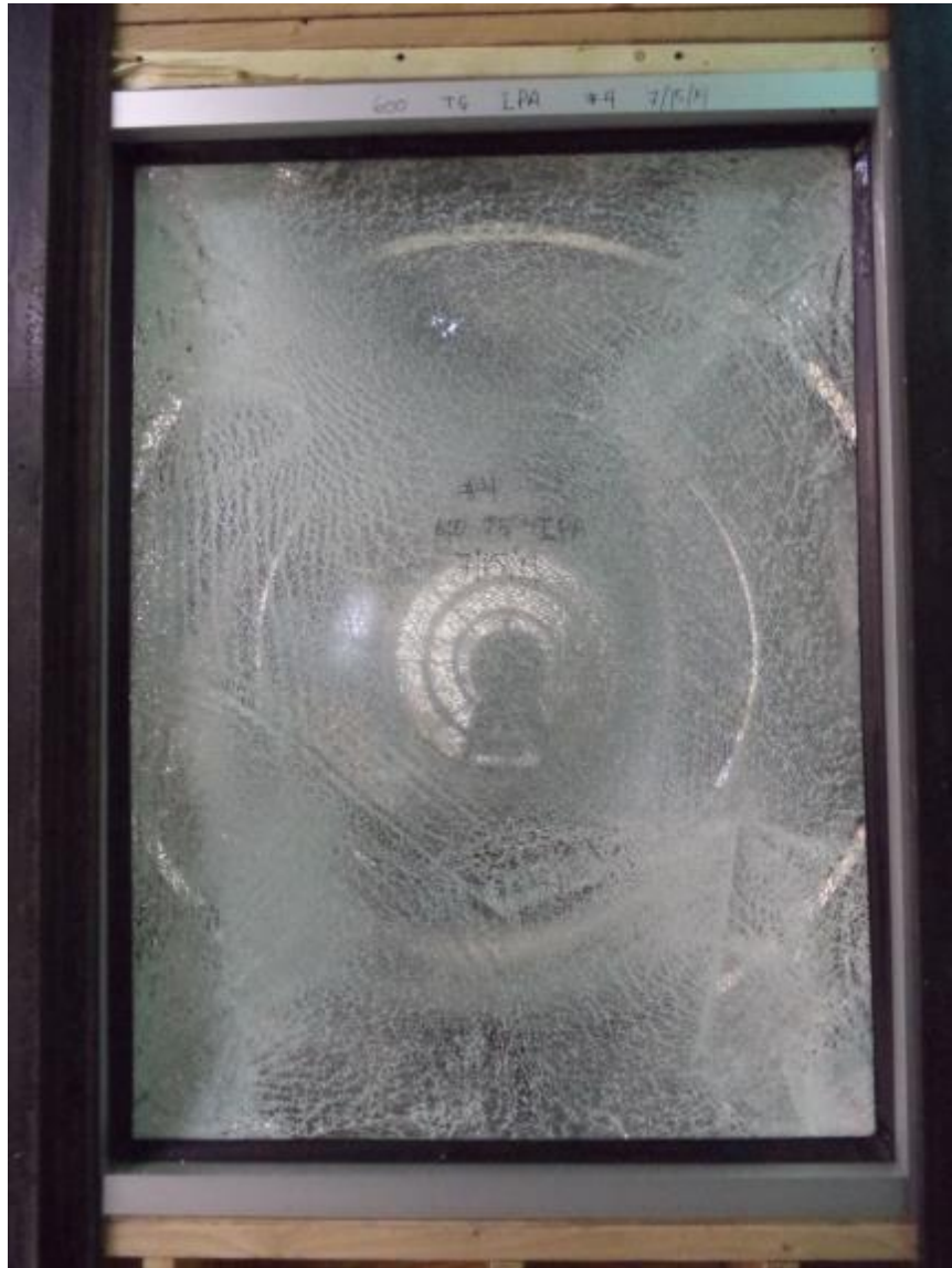
Photo No. 6 Post-test Specimen #2, Interior
