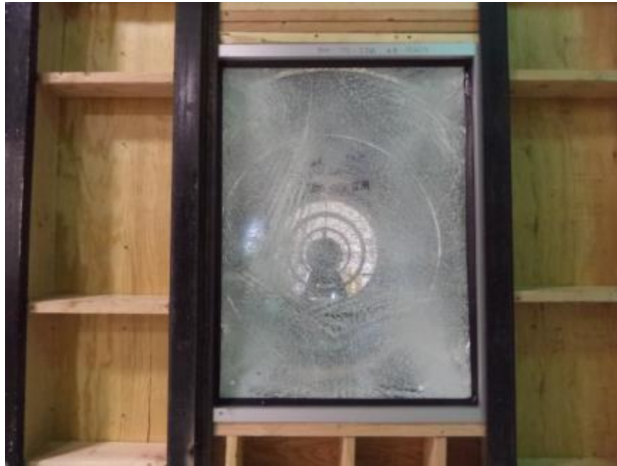
Photo No. 14 Post-test Specimen #5, Interior
