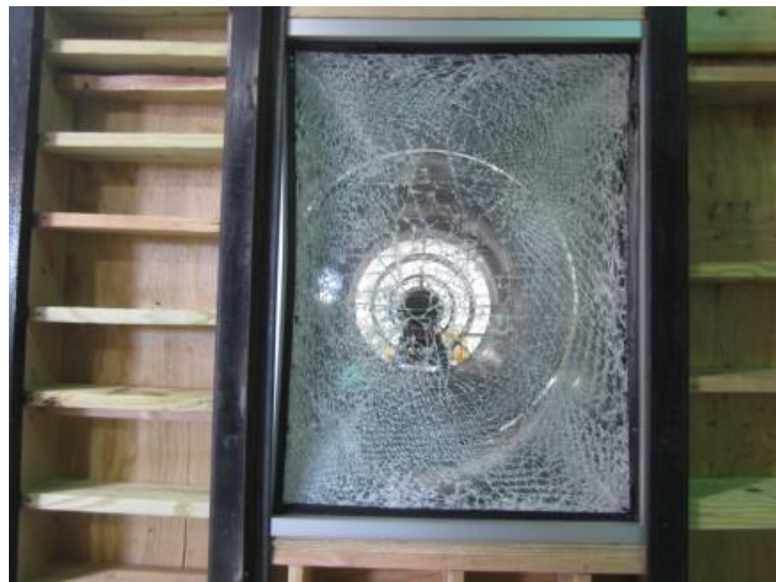
Photo No. 40 Post-test Specimen #15, Interior
