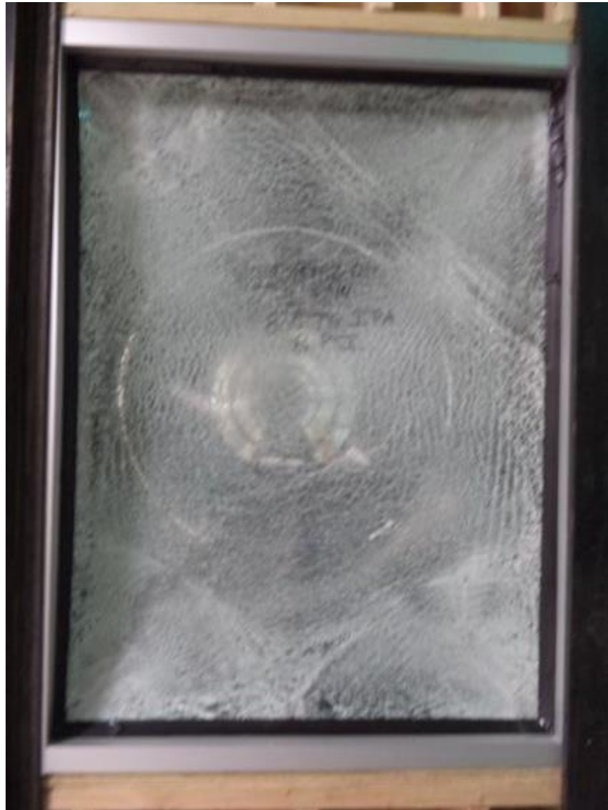
Photo No. 22 Post-test Specimen #8, Interior
