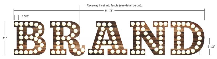
One (1) Set of Exposed Bulb Illuminated Channel Letters on Raceway
